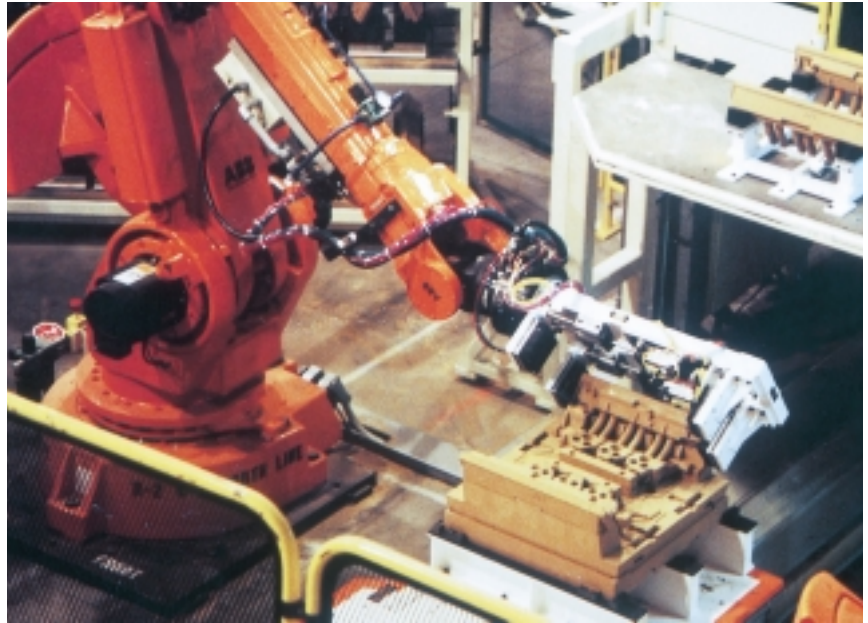
3 Special wrist of a robot developed for applications in foundries. It can withstand mould sand, dust, sprayed liquids and high temperatures.
