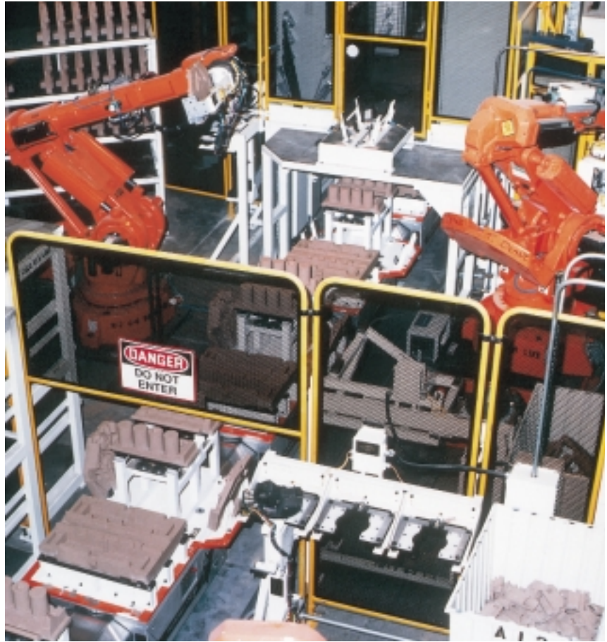
Assembly of sand moulds at Ford Windsor, Canada. The mould assembly is progressively built up on a pallet, which is transported on a rail car to the robot cells. 6
