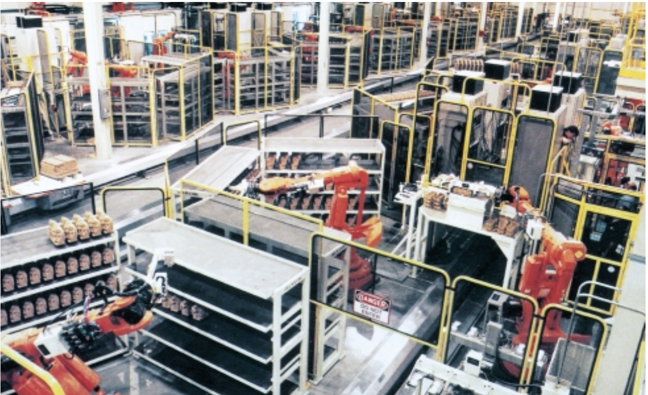
5 Aluminium foundry at Ford Windsor, Canada. The foundry is one of the most advanced fully automated plants of its type in the world. More than 100 articulated-arm and gantry robots from ABB Flexible Automation produce cylinder blocks and heads for a range of Ford engines.
