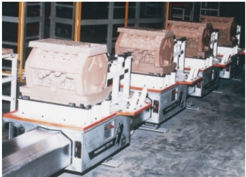
Sand moulds weighing up to 200 kg are transported on pallets in the foundry. 7
