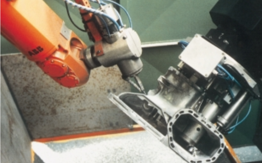
Robots are highly versatile and can be easily reprogrammed to carry out a new operation, such as deburring.
