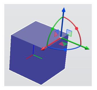
When moving or rotating an object the offset from the start position is displayed next to the axis. It is also possible to manually type in an offset.
