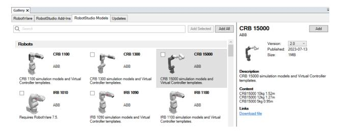
Model packages can also be installed on-demand from the ABB Library menu or when creating a new Virtual Controller. A model that is not installed is indicated by a download symbol.
