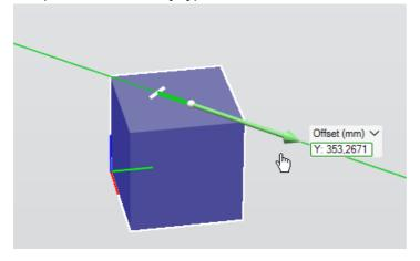
Select the "Reference" option in the dropdown menu to show the position relative to the selected reference coordinate system, instead of the offset from the start position.
