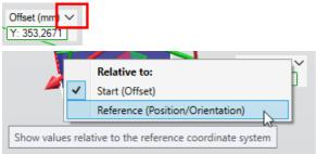
Press the Ctrl key when moving or rotating to snap to increments. Press Ctrl+Shift to snap to fine increments. For linear movement the size of the increments depends on the zoom level. For rotation the increments are 5 degrees and the fine increments are 1 degree.
