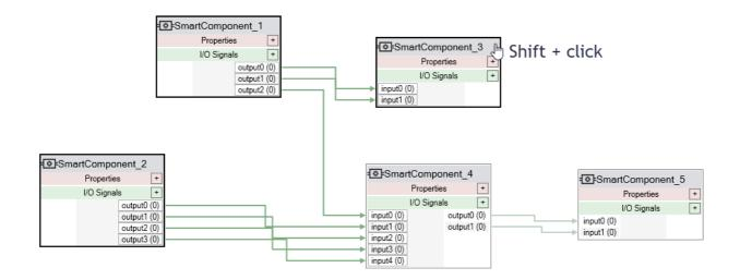
Multiple Smart Components can also be selected by clicking on the background and dragging a selection rectangle around the Smart Components. If the SHIFT key is pressed while rectangle selecting, the selected Smart Components are added to the current selection.
