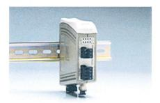
The ODW-710-F2 is designed for harsh industrial usage as well as road or railway installations meeting industrial level EMC specifications and having a wide operating temperature range. It is able to automatically detect the data rate of the connected PROFIBUS DP device and hence needs minimal configuration prior to use. The unit also has a re-timing function that eliminates the problem of jitter and hence ensures reliable communications in all situations.
