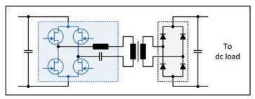
Figure 3: LLC resonant converter using GaN
