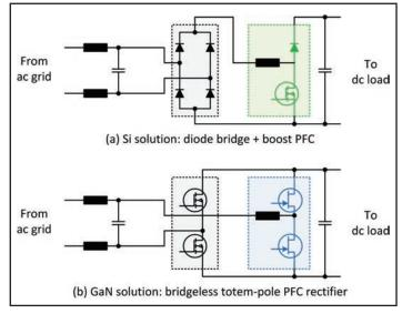
Figure 2: PFC rectifier using (a) Si; (b) GaN.
