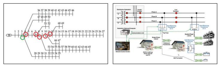
Fig.2 Schematic showing proposed installation of concept auto-balancing transformer (green) as replacement of one of the conventional distribution transformer (red) | Fig.3 Field demonstration scenarios
