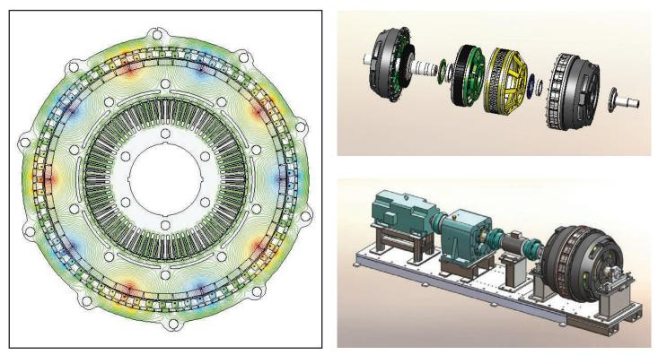
Figure 2: Electromagnetic simulation of the full generator. | Figure 3: exploded view of generator. | Figure 4: Test bench with drive machine (left) and generator (right). Gear box and torque transducer are also shown
