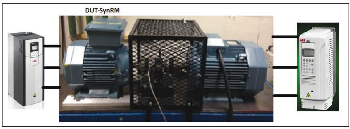
Figure 1: Experimental Setup: SynRM driven by an ABB low voltage (LV) AC drive coupled to an IM
