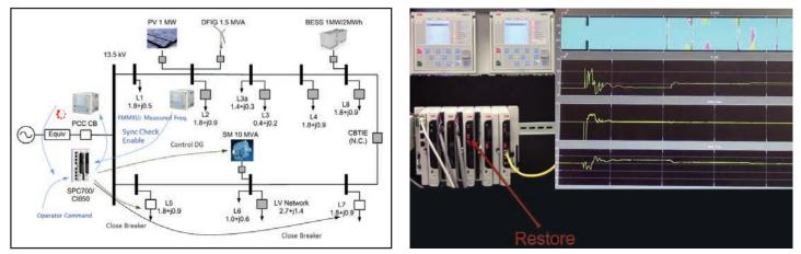
Figure 1: Integrated microgrid protection and control functions for resynchronization. | Figure 2: HIL Simulation results – unplanned islanding and resynchronization.
