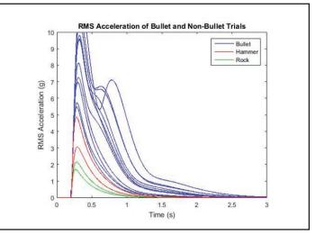
Figure 1: Impact on a test object during a UL-9 trial | Figure 2: RMS acceleration for bullet trials
