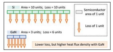
Figure 4: Illustration of the thermal management challenge with GaN
