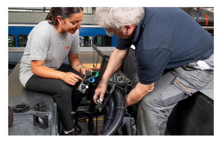
Possible ways of using the new modular support system BGPM, are discussed with customer. The BGPM is a light, compact solution offering high impact resistance. The external dimensions of this new design have been reduced to the minimum and the spacing between parallel conduits is very small. The system has been specially designed for use in the rail vehicle construction sector and for other applications where conduits and cables running in parallel need to be held in position.
