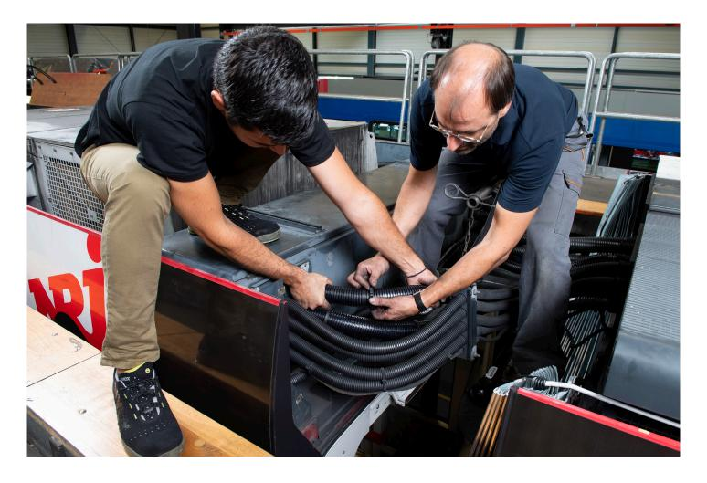
The divisible PACOF conduit can be quickly and easily fitted over the damaged area, helping guarantee total protection piece, provides IP54 protection, quick and easy to assemble, suitable for retrofitting and repair tasks, of a modern functional design, of high quality, and an excellent value for the price.
