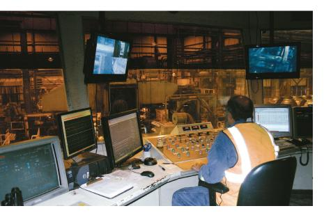
Steelscape's 4-hi single stand reversible mill running with a Stressometer 7.0 FSA system, controlling the flatness on both entry and exit sides.
