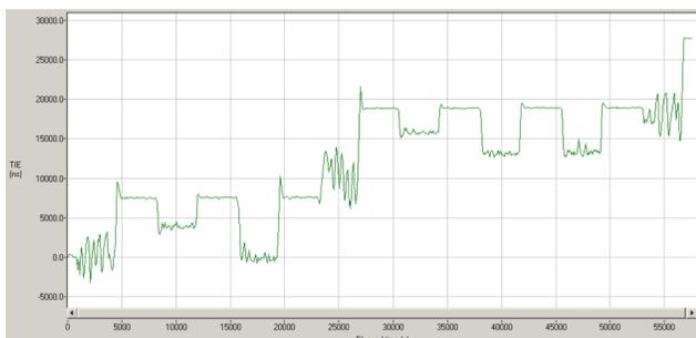
Figure 3: Accumulation of long-term residential jitter buffer delay depending on traffic pattern
