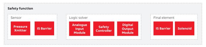
In the example above, it can be seen that the SIS comprises of three subsystems and seven devices:
