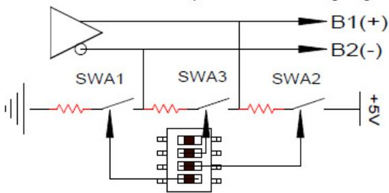
**SWITCH B:** used for serial parameters and principal functioning possibilities
