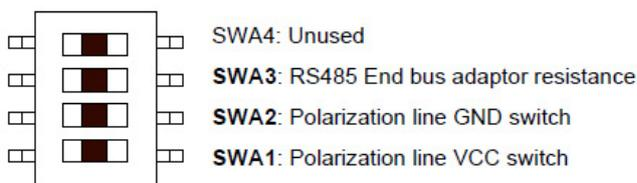
The on position is on the left side of the switch (keeping orientation of the previous figure)
