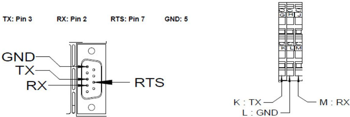
This configuration can replace any serial PC connection with an Ethernet connection using e-ILPH and the same cable used before. E.g. with AC31, any CPU can be connected to the serial port using standard 07SK50 cable
