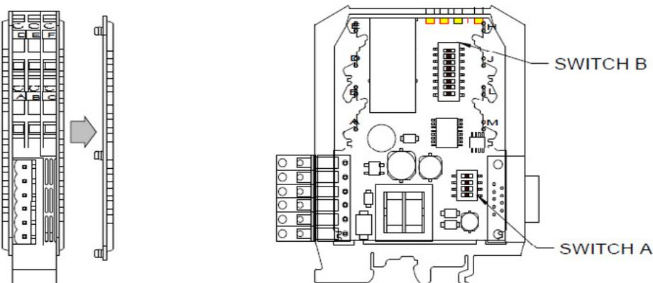
**SWITCH A:** used for hardware configuration of RS485
