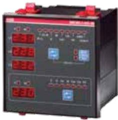
The DMTME-I-485, DMTME-I-485-96 and DMTME-I-485-72 models are additionally equipped with two digital relays, fully programmable as either pulse outputs for remote metering of energy consumption, or as alarm outputs. The output relay can be set as NO or NC.
