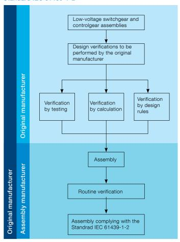
One can also observe that the standards is very stringent when it comes to design verification is IEC 61439. Design verifications are required to be carried out only by OEM manufacturer. Assembly manufacturer is not authorized to implement any design changes.
