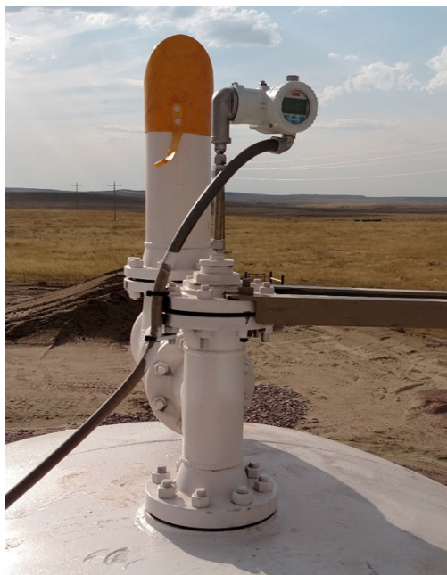
LMT100 for safe and reliable level measurement
