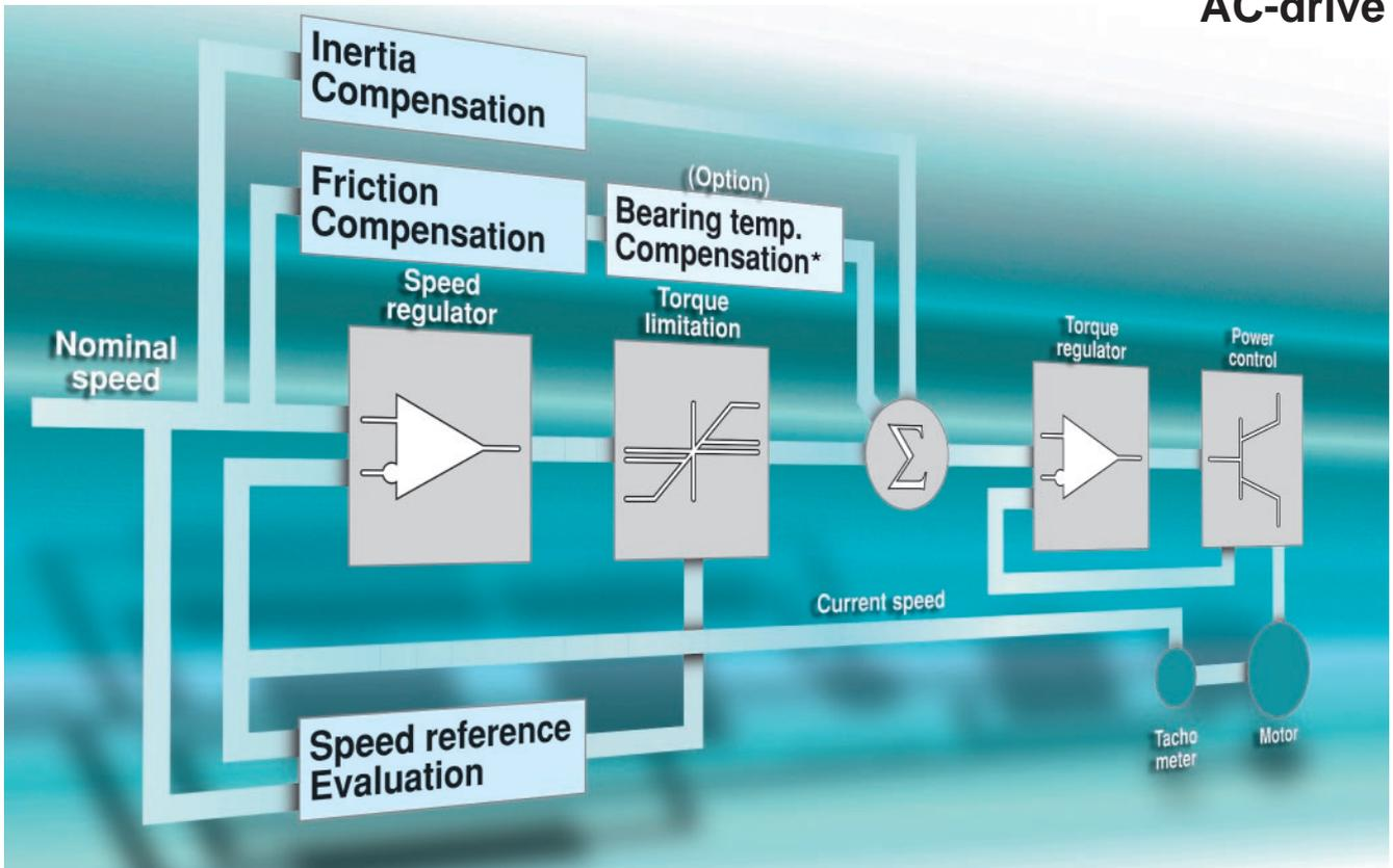
The picture above describes the function of the special Stressometer drive application. The gray boxes describe a normal roll drive system.
