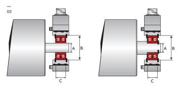
Note: Bearing specifications in table are samples. PRT load cells can accommodate bearings for many other shaft diameters besides those shown.
