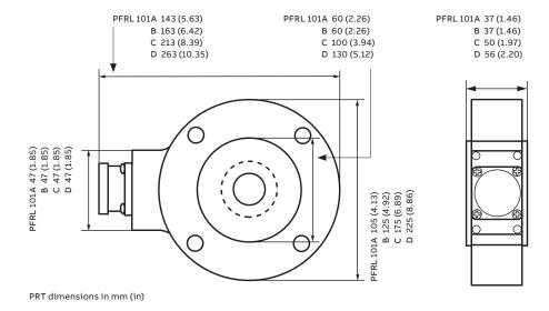
Designed to measure web tension on most types of web processing machinery used in the converting, plastic film, printing, textiles, and other industries.
