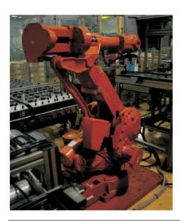
Mett has more than 50 robots, used for everything from machine tending to sawing, deburring, ladling, palletising, gluing, assembly work and cleaning.
