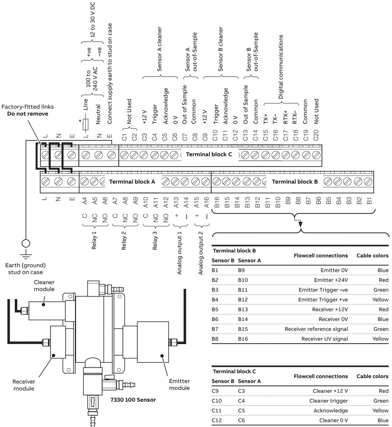
\* 500 mA type T fuse (AC) or 4 A type T fuse (DC)
