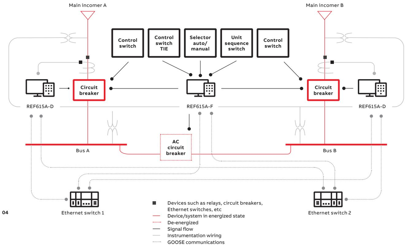
04 Typical single-line diagram of an M-T-M ATS configuration.
