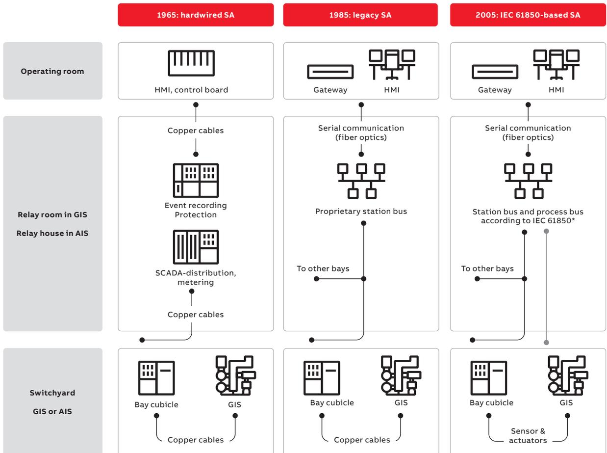
\* The process bus is not a must in IEC 61850 but only an option
