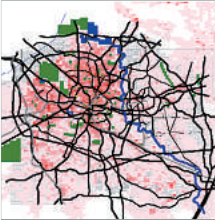
Load forecast study performed using a commercially available GIS database as starting point
