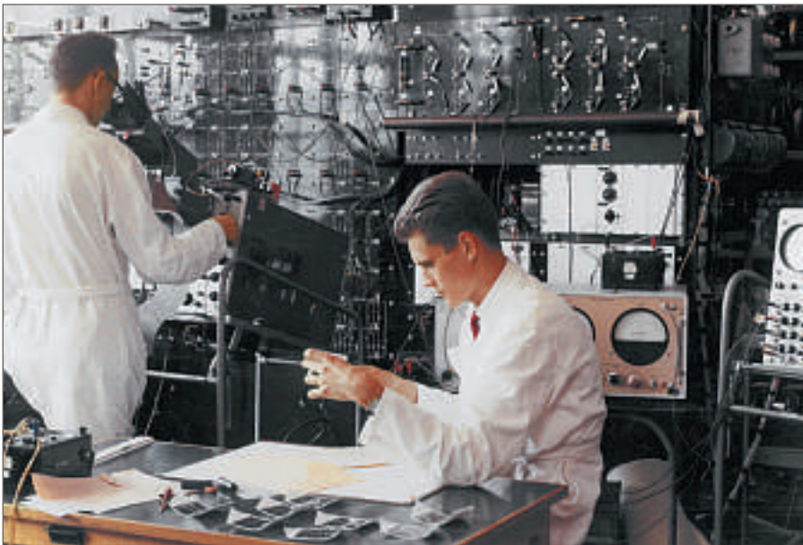
Analog simulator used in the design of the early HVDC transmission systems
