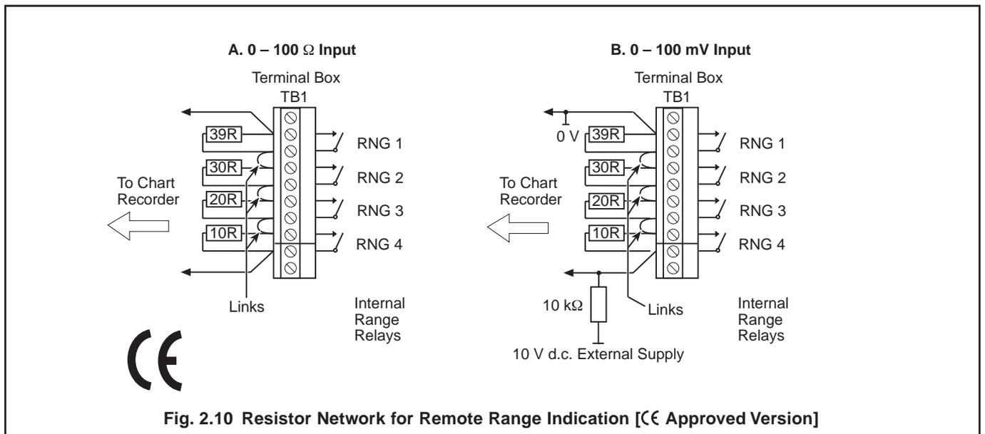
**Fig. 2.10 Resistor Network for Remote Range Indication [CE Approved Version]**
