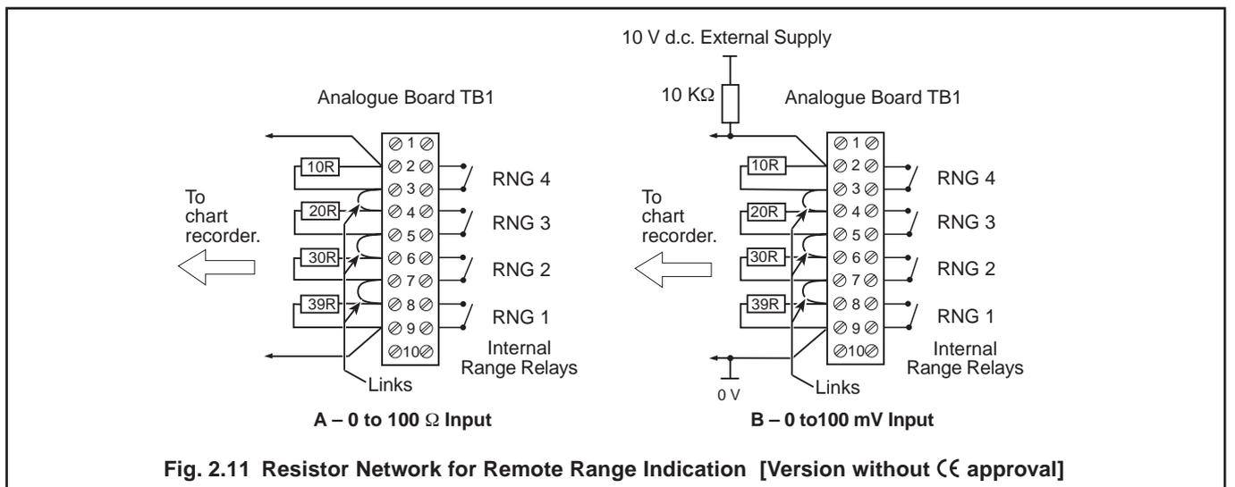
**Fig. 2.11 Resistor Network for Remote Range Indication [Version without CE approval]**
