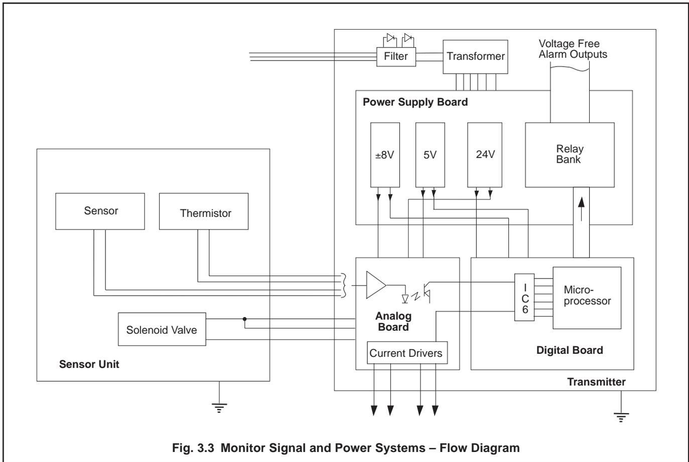
Fig. 3.3 Monitor Signal and Power Systems – Flow Diagram
