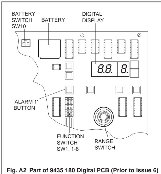
**Fig. A2 Part of 9435 180 Digital PCB (Prior to Issue 6)**
