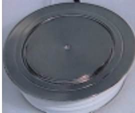
Power electronic components can easily switch over 3000 A hundreds of times per second.
