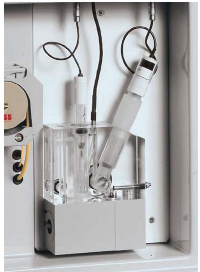
Multi-channel Peristaltic Pump and Sensor Flow Cell
