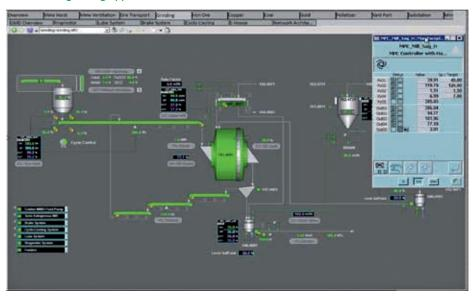
hibits relatively long time delays related to the slow transport of the raw meal along a series of heat exchangers, cyclones and then the kiln.
