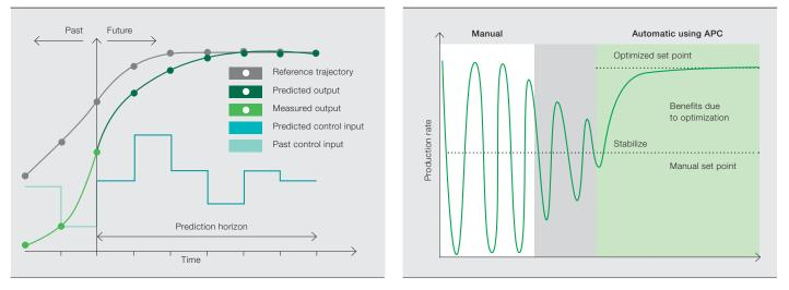
Using the square form in the objective function serves to make the control problem "well behaved."
