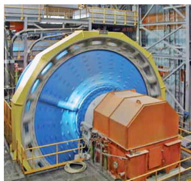
View of the SAG mill (3,360 kW) at Agnico-Eagle’s LaRonde mine.
