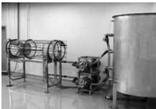
Basic set-up during construction. Separator (left), pumps, reservoir tank and flexible hosepipes.
