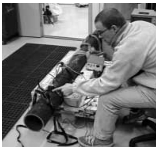
A scientist checks an instrument during a feasibility study on an ultrasonic pipe-length meter.
