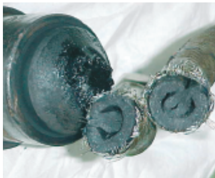
Figure 3. Blocked water cooling tube.
