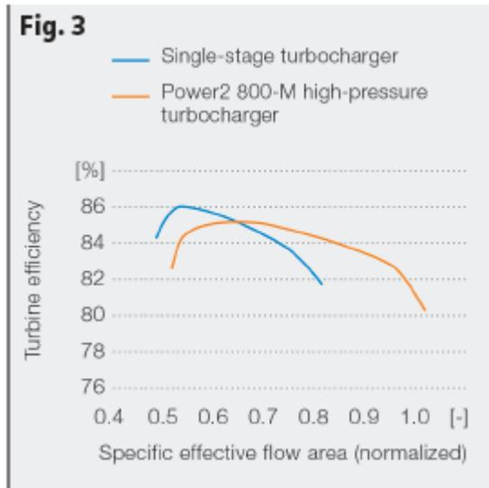
**Fig. 3:** Turbine efficiency vs. specific effective flow area of a single-stage turbocharger and Power2 800-M high-pressure turbocharger.
