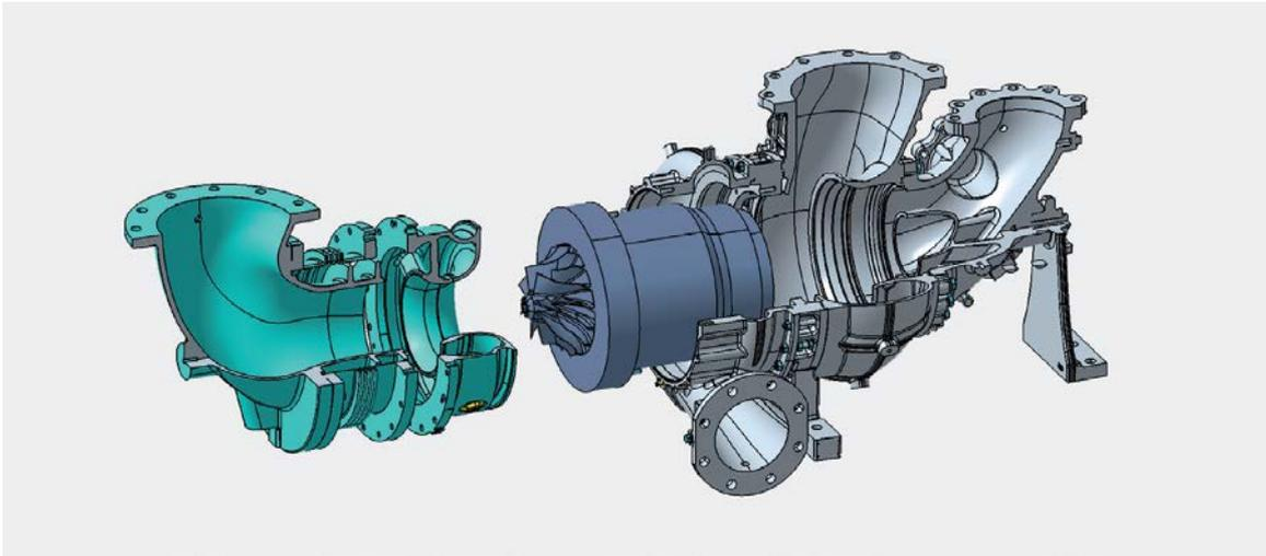
**Fig. 5:** Power2 800-M high-pressure turbocharger with extractable cartridge.
