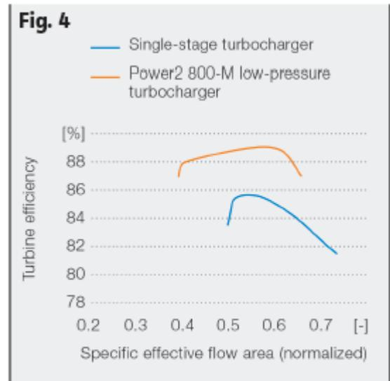
**Fig. 4:** Turbine efficiency vs. specific effective flow area of a single-stage turbocharger and Power2 800-M low-pressure turbocharger.
