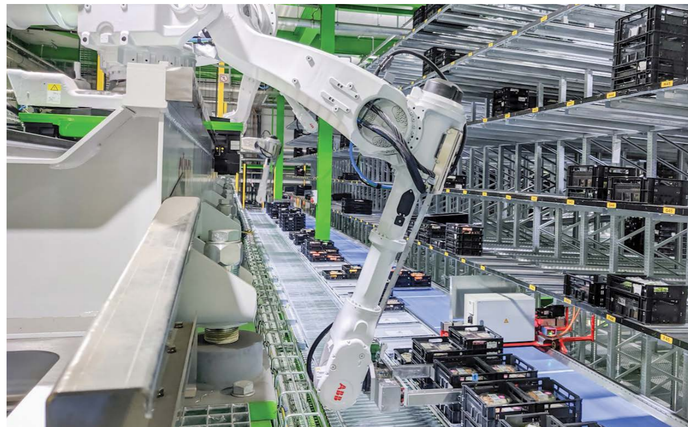
A robotic order picking installation at Heemskerk's Rjinsburg facility in the Netherlands prepares orders according to each supermarket or food retailer's needs, so that the products can be cross docked directly onto supermarket shelves instead of being stored at distribution centers.
