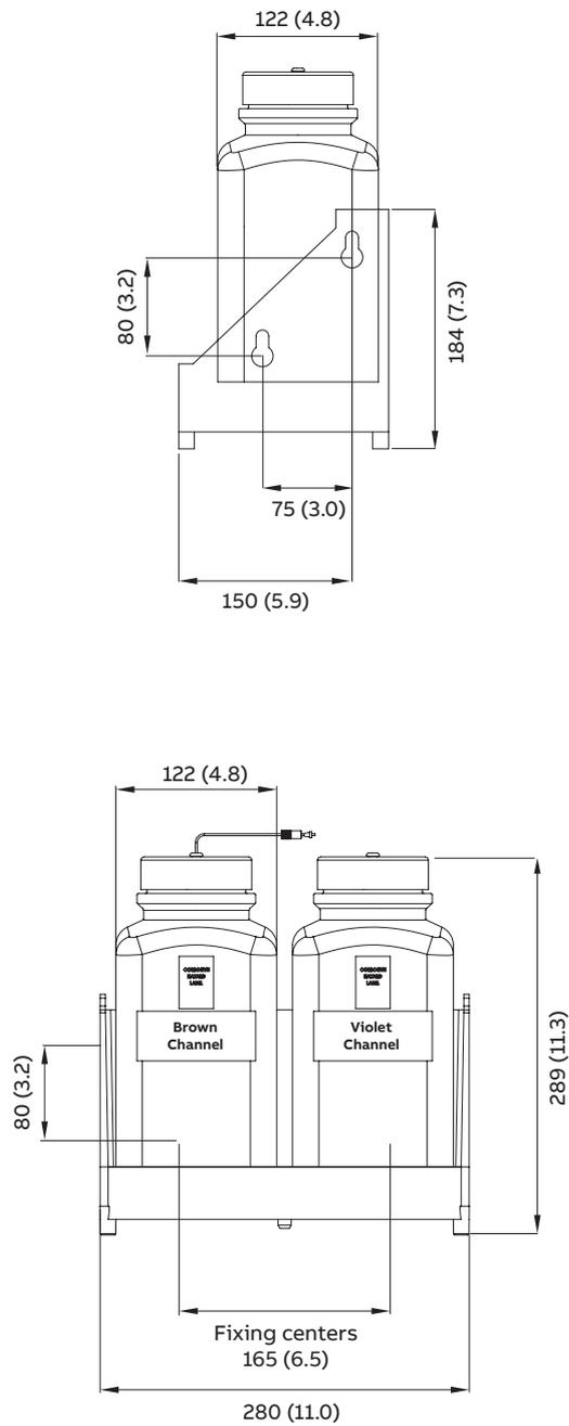
Figure 7 Reagent bottles mounted on optional bracket
