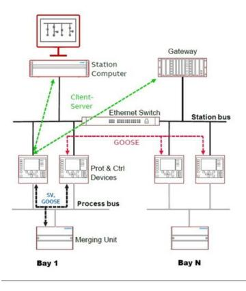
Thanks to IEC 61850-8-1 part which allows the elimination of copper wires between relays on horizontal level i.e. relay-to-relay communications substation bus & IEC 61850-9-2LE which allows sharing of digitized information from instrument transformers or sensors in a standardized way to other relays- process bus. These services are classified as:
