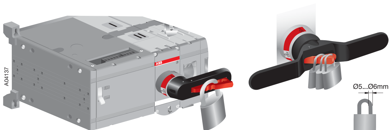
Figure 3.4 Locking the manual operation
