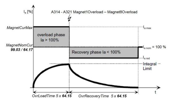
Up to 8 magnets can be monitored with I<sup>2</sup>t accumulators:
