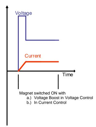
The diagram above shows how the magnet current reference can be reached as quickly as possible after start command of the converter. Voltage or current control can be used.
