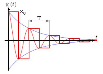
There are requirements of erasing the remanence of magnets completely. The operation mode which is called **Degaussing by pulsing** is shown in the diagram above. Decreasing and alternating the magnet current will erase the residual force.
