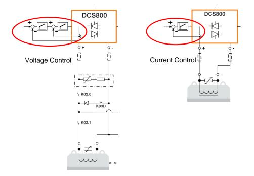
Magnetic force can be dynamically increased and decreased using pure current control using the full voltage range. But a longer pure current control can overheat the magnet. Magnets in parallel prefer voltage control. This will prevent possible overloading of the individual magnet. Depending on the requirements, a combination of current and voltage control is desirable.
