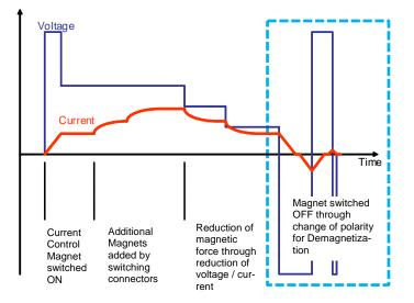
Demagnetization or Degaussing Mode (Selection in parameter 60.15):
