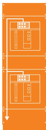
SACE Emax 2's design and performance in a switchboard allows for significantly reduced footprint for switchgears. In addition, the integrated Ekip Touch trip unit and on board Ekip Com Modbus module ensure the accuracy of measurements and connectivity with the communications network.
