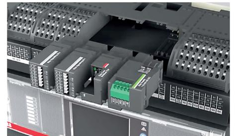
The Ekip Com modules enable all SACE Emax 2 circuit-breakers to be integrated into an industrial communication network for remote supervision and control of circuit-breakers without the need for external interface devices. They are mounted within the terminal box, which means that communication can be maintained with withdrawable circuit-breakers, even while in the racked-out position.
