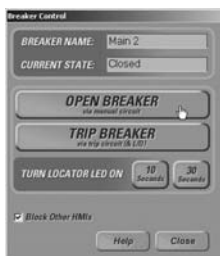
Figure 13.6 Breaker Control Window for Circuit Breaker Main 2
