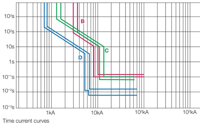
Figure 4 shows how it is possible to switch to a set of parameters which guarantees selective coordination between circuit breakers C and B by means of the “dual setting” function.
