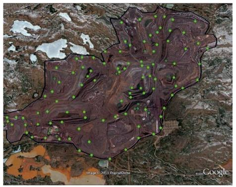
With the ABB Tropos wireless mesh networks, routers deployed on trailers around the pit "discover" each other automatically and provide ubiquitous coverage for the entire pit.
