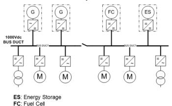
Figure 5 – ABB's DC Grid single line diagram
