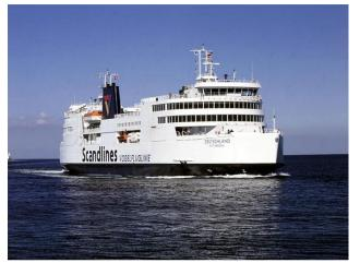
Figure 7 - M/V Deutschland recently retroffited with batteries as main power source
