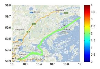
Figure 9 - Number of generators running with batteries as spinning reserve
