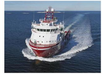
Figure 6 - PSV "Dina Star" equiped with DC electric propulsion
