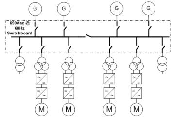
Figure 4 - Traditional AC system's single line diagram
