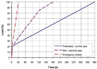
Figure 10 - Maximum load increase rate for engines operating at nominal speed
