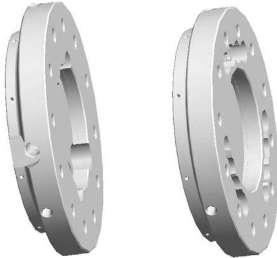
Figure 13 Seven holes on a radius of x mm from axis 6 center on the two standard tool flanges.
