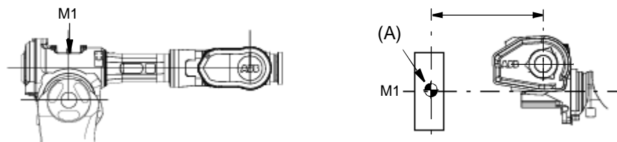
Figure 29 Permitted extra load on upper arm.
