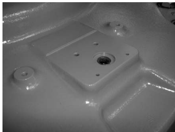
Figure 12 One \text{\O}12 H8 (depth 12) in +- direction from axis 1 center of robot base.
