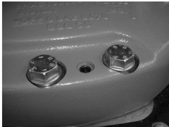
Figure 11 Four \text{\O}12 H8 (depth 12) on radius 400 mm from axis 1 center on robot base.
