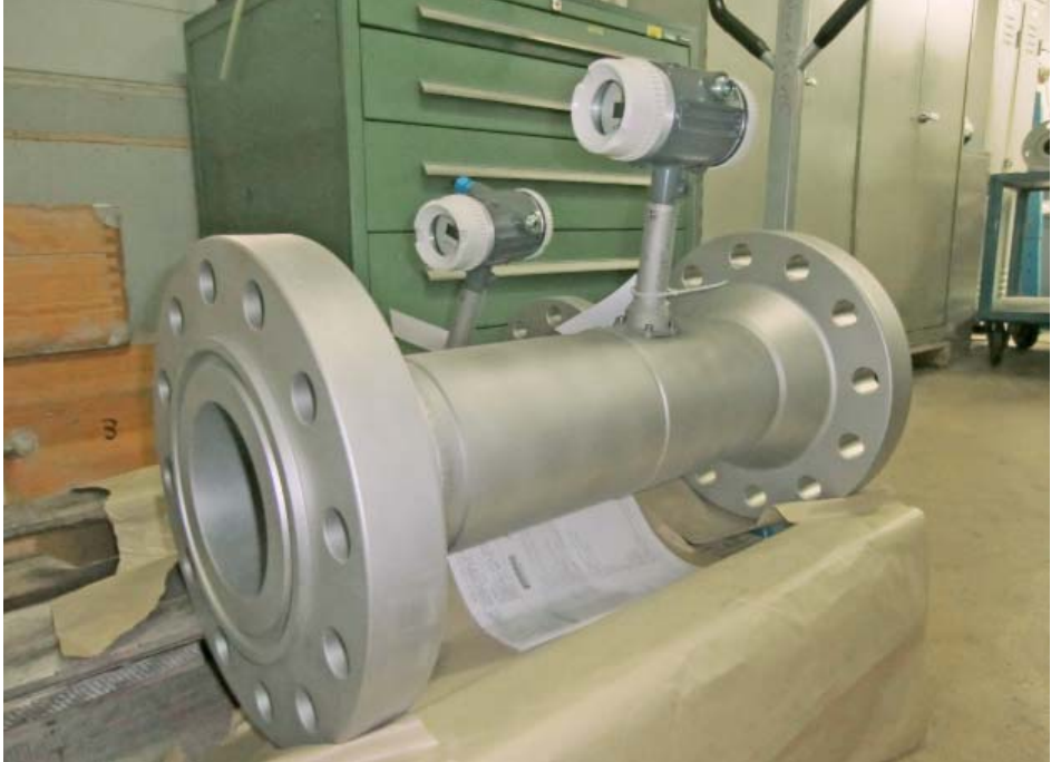
6" (DN150) swirl flowmeter with ASME class 900 RTJ flanges
