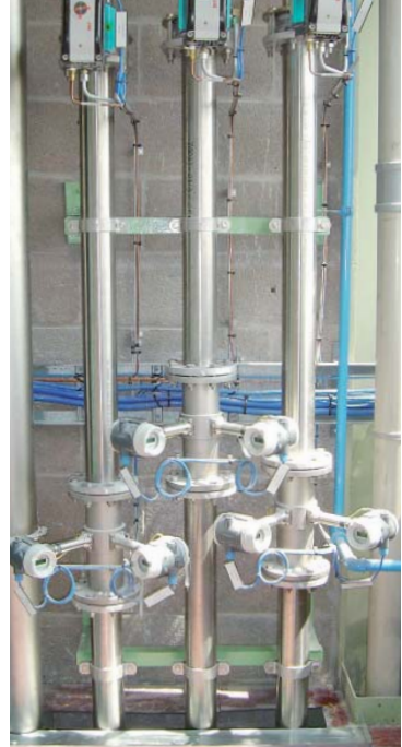
Dual sensor swirl flowmeter with 120° sensor layout
