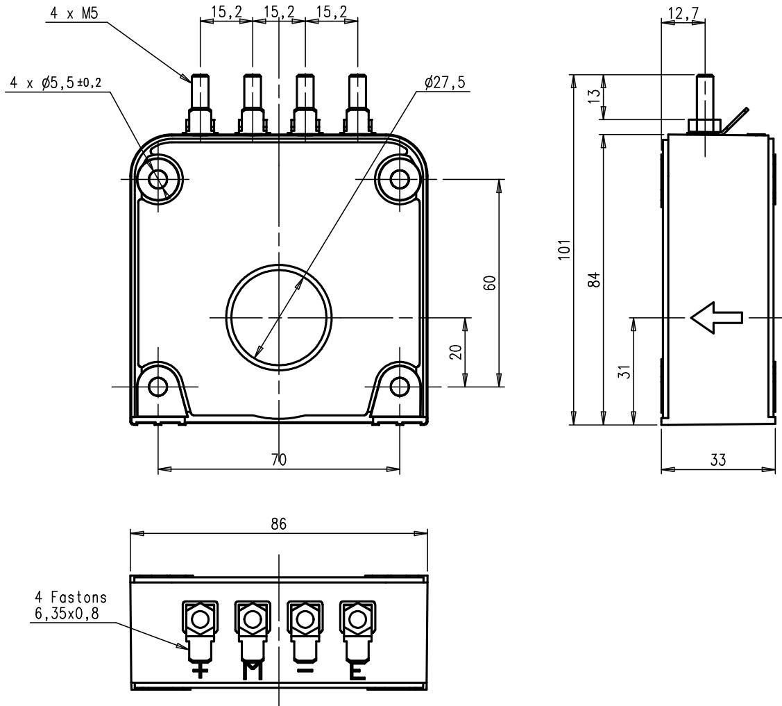
**Maximum M5 tightening torque: 2 N.m**
