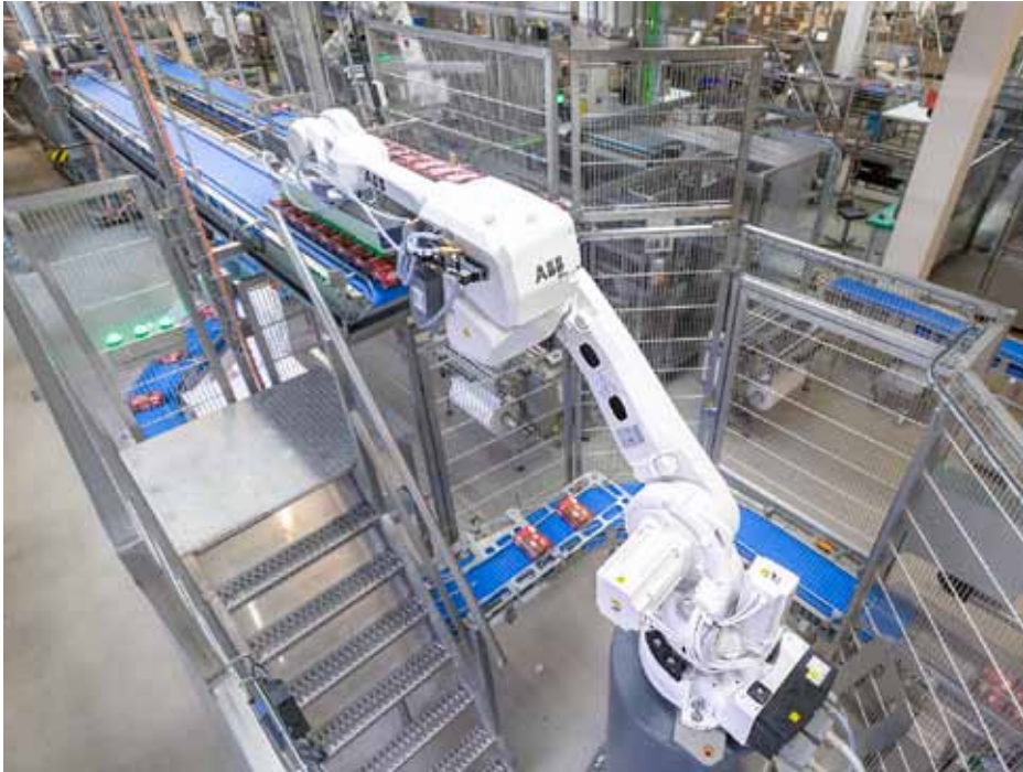
One of four ABB IRB 360 robots packaging frozen dessert products.
