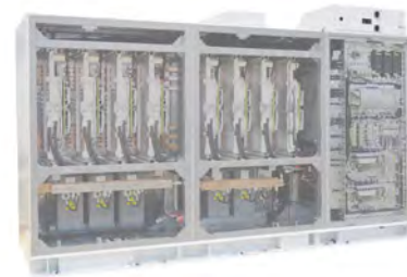
Compact Converter 3 MW for electric locomotives
