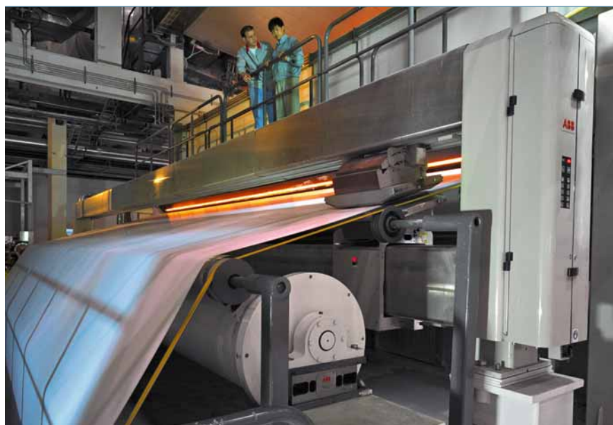
1 Network Platform scanning with high-temperature cover
