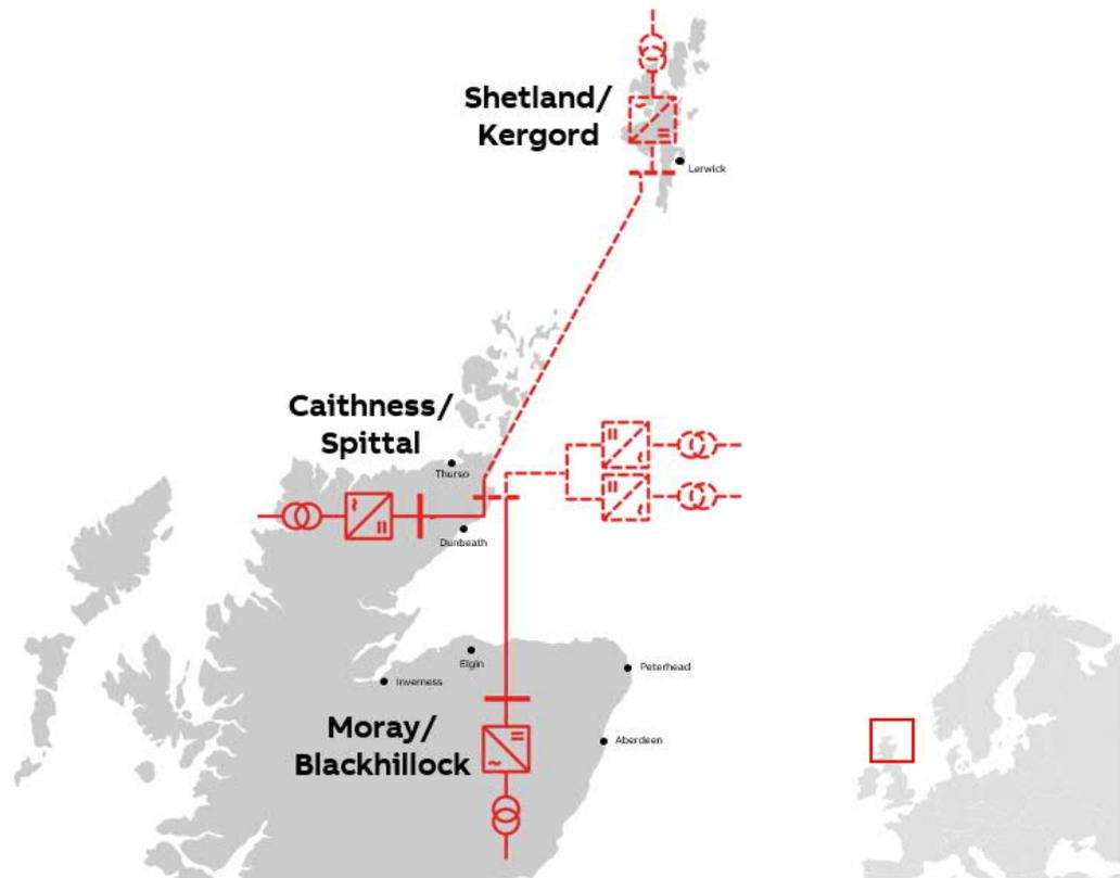
Figure 8. Caithness Moray HVDC Link in northern Scotland is designed for a five terminal HVDC system (straight lines). The foreseen extension is shown with dashed lines, where the DC switching station is at the midpoint for the multiterminal system shown as a dashed busbar.
