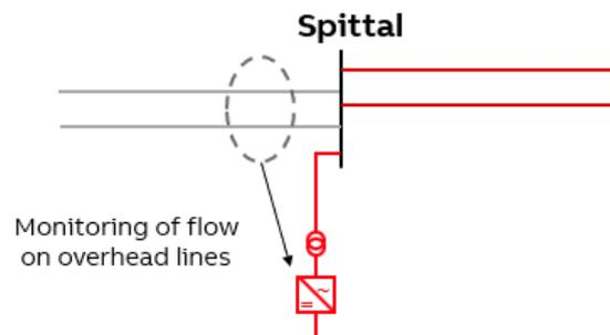
Figure 7. The HVDC control system in the CM HVDC link monitors the power flow on the 132kV circuits PM1 and PM2 and acts with APOL or EPC.
