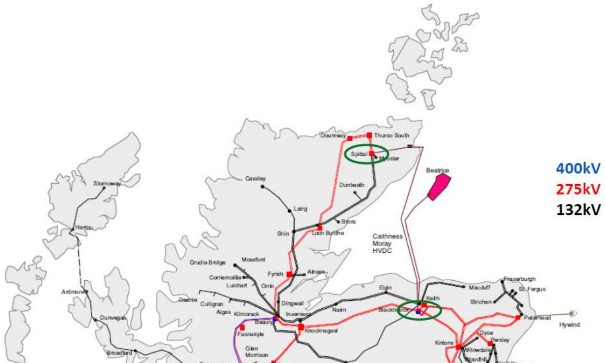
Figure 3. Overview of the 275kV AC transmission corridor in parallel with the CM HVDC link, together with the 132kV circuit. Both converter stations, Spittal and Blackhillock, encircled with green.
