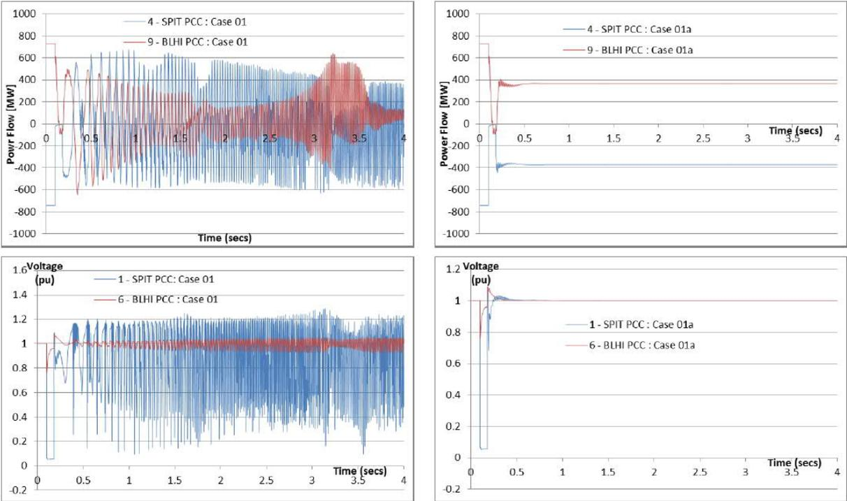
Figure 6. The two left-hand graphs showing a voltage collapse without EPC, and the right-hand graphs showing a successful run-back.
