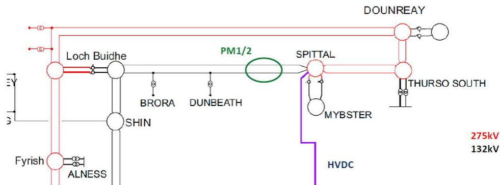
Figure 4. The 132kV double circuits, PM1 and PM2 connection into the Spittal station together with the 275kV double circuits transmission corridor, where the substations are marked as circles
