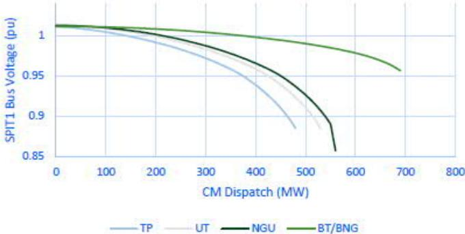
Figure 5. PV analysis exploring different outages and converter dispatches.
