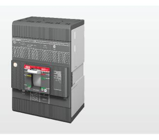
225 A frame available up to 480 V Delta UL. Thermal-magnetic, MCS and MCP trip units. Max. interrupt rating of 35 kA at 480 V. Reliably covers 480 V applications. Rated for 25,000 mechanical operations.
