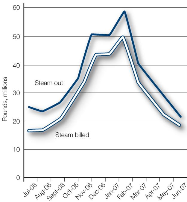
New ABB swirl flowmeters FS4000 have closed the gap between steam delivered and steam billed at Virginia Commonwealth University
