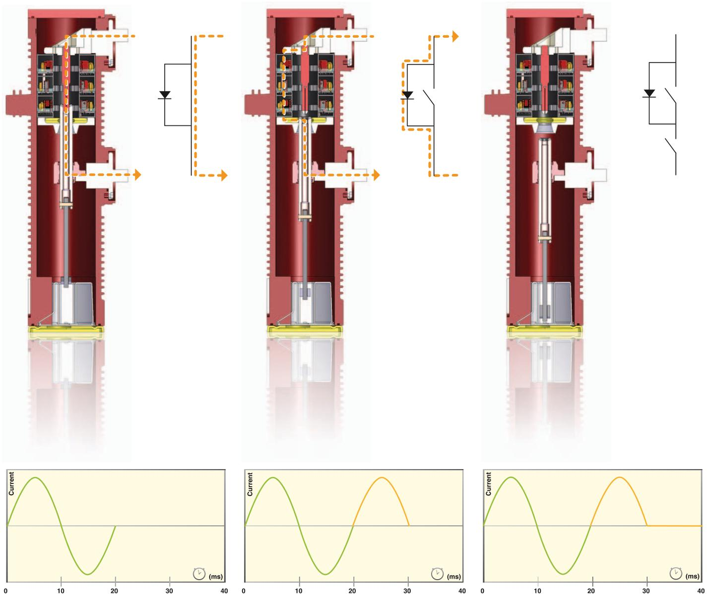
Switch in close position, capacitor bank is connected to the distribution network.
