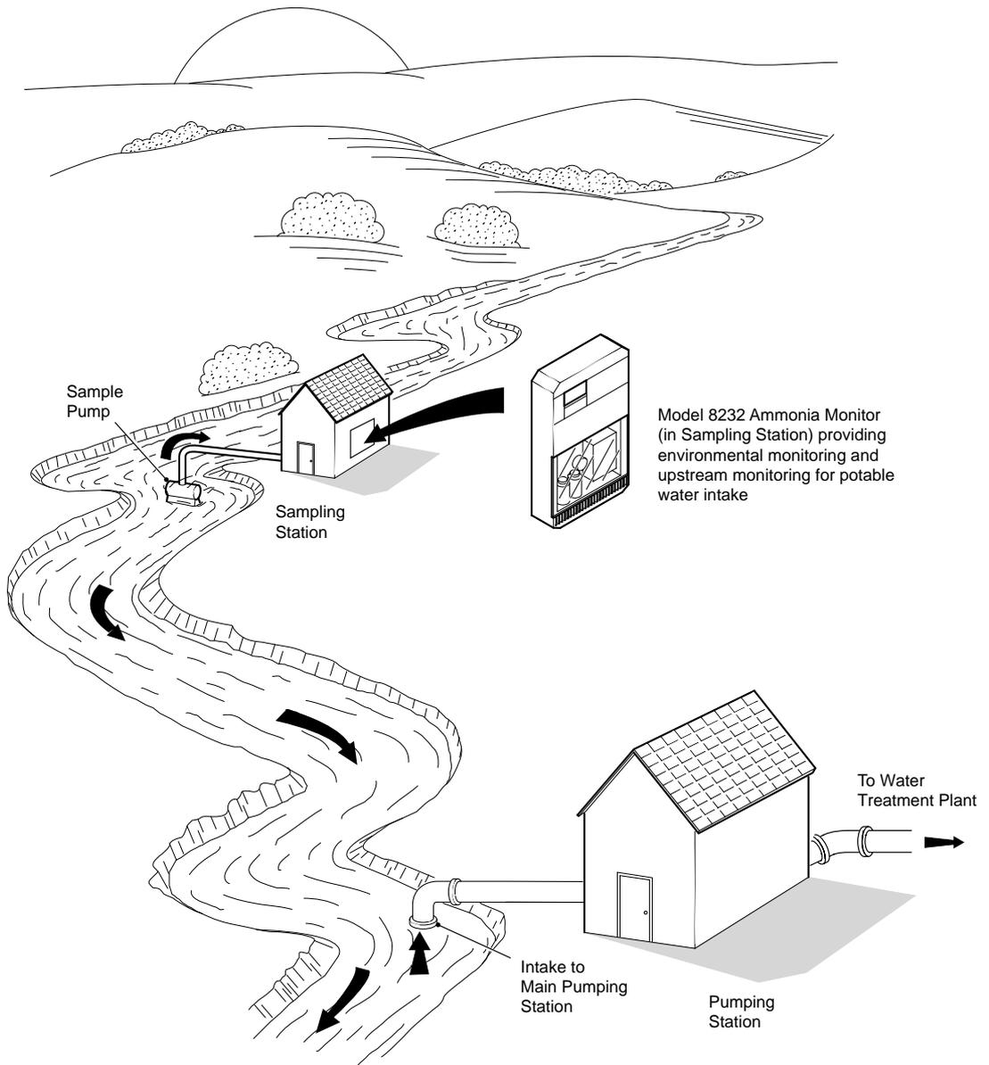
At the sampling point, a sample is drawn from the river via a pump and ultrafiltration system and pumped to the type 8232 Ammonia monitor as shown above.
