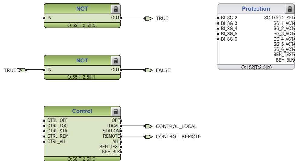
Figure 114: Functions for general logic states TRUE and FALSE, protection setting group selection and local and remote control
