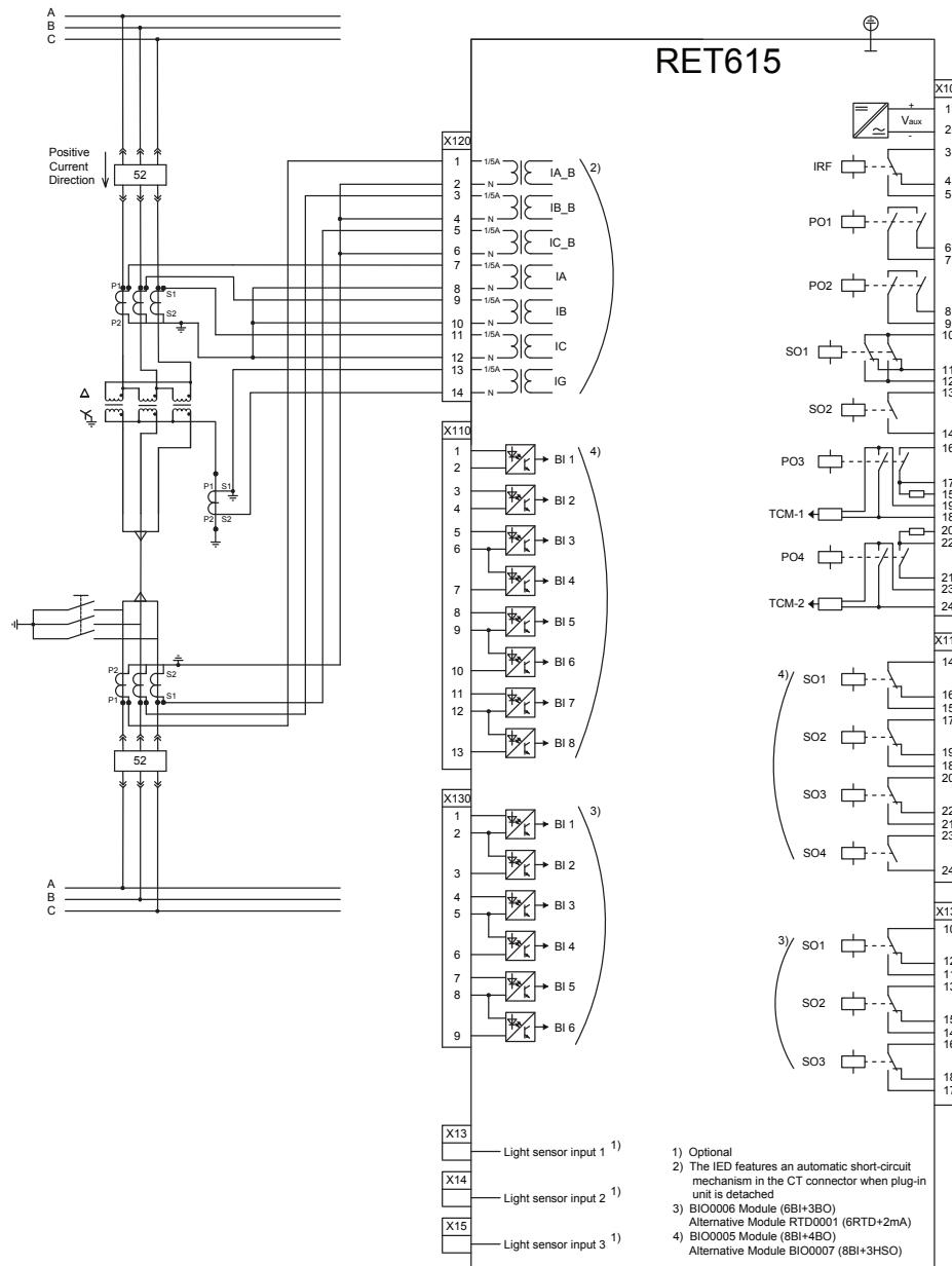
Figure 9: Connection diagram for the B configuration
