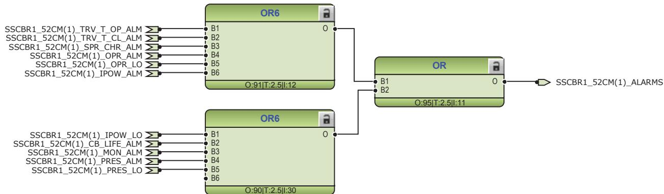
Figure 82: Logic for circuit breaker 1 monitoring alarm
