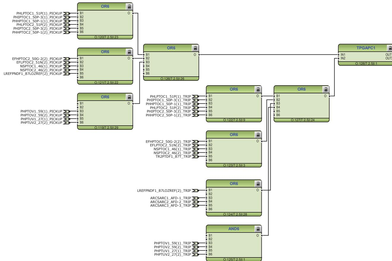
**Figure 75:** General pickup and trip signals
