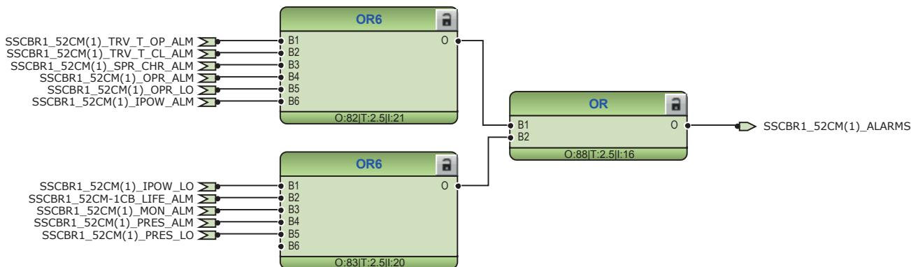
**Figure 29:** Logic for circuit breaker 1 monitoring alarm
