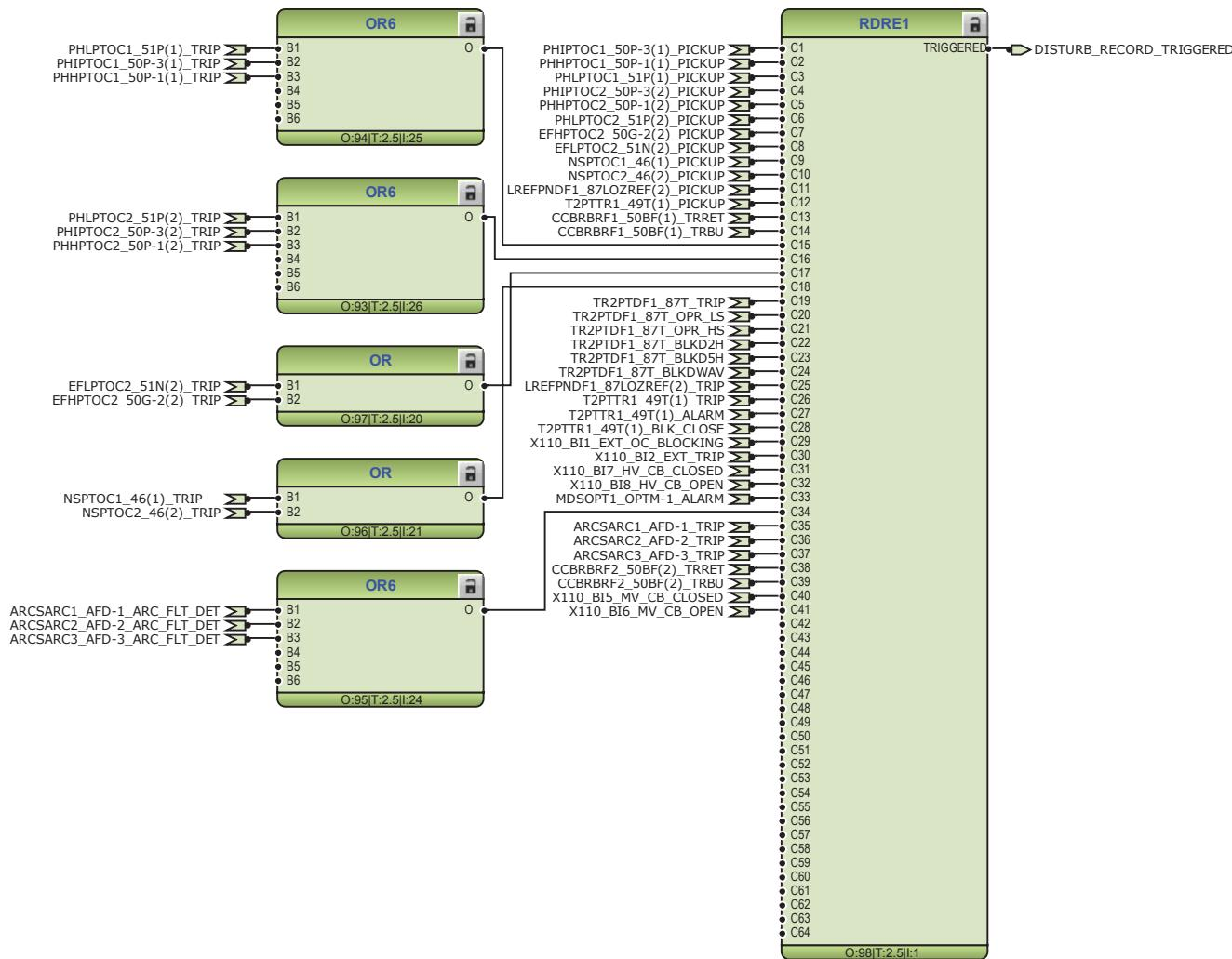
Figure 26: Disturbance recorder
