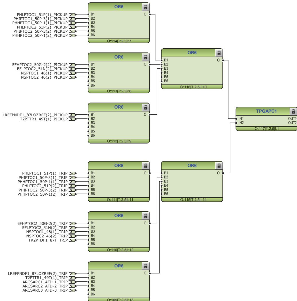
Figure 23: General pickup and trip signals
