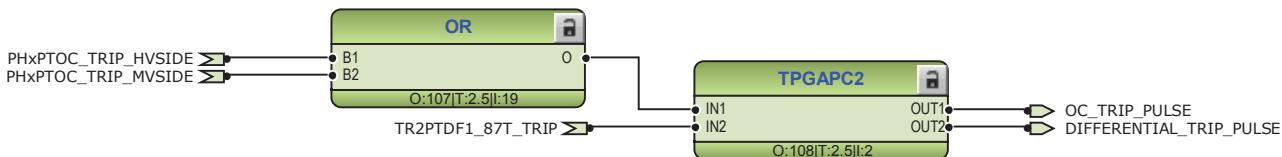
Figure 58: Timer logic for overcurrent and differential trip pulse
