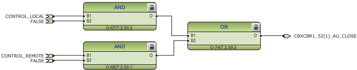
Figure 93: External closing command for circuit breaker 1
