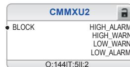
Figure 45: Current measurement: Three-phase current measurement (MV side)
