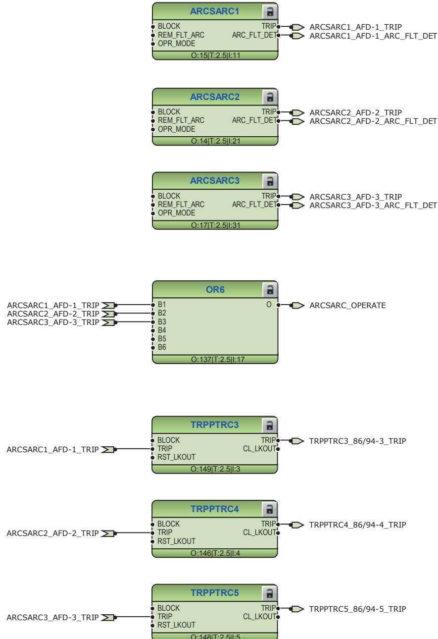
Figure 73: Arc protection with dedicated high-speed output
