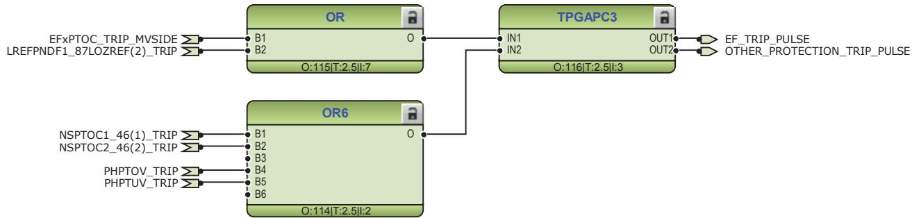
Figure 116: Timer logic for ground-fault and negative sequence with thermal overload protection trip alarm
