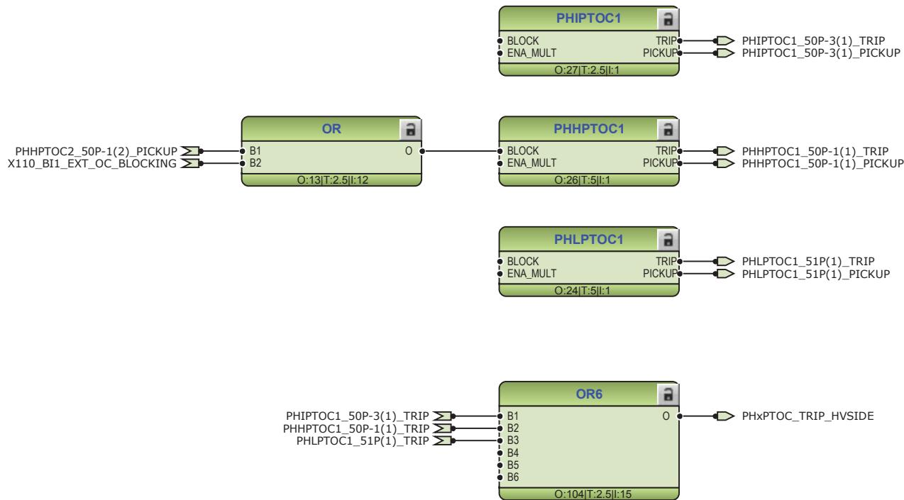
Figure 13: High-voltage side overcurrent protection function
