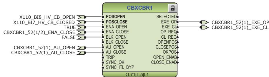
Figure 32: Circuit breaker 1 control logic
