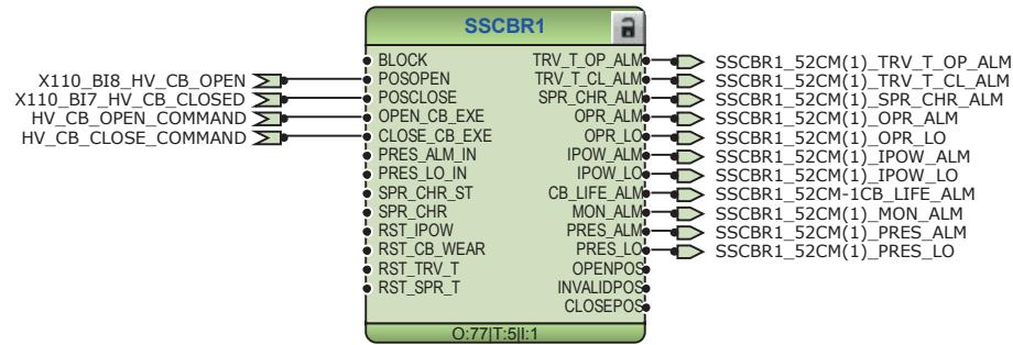
Figure 27: Circuit-breaker 1 condition monitoring function
