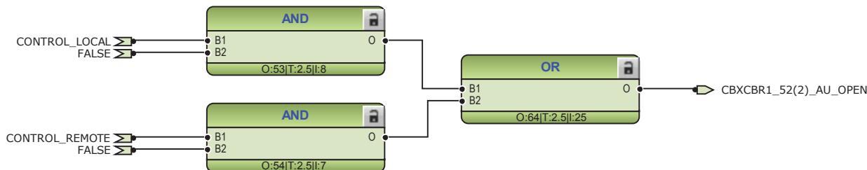
*Figure 42: External opening command for circuit breaker 2*
