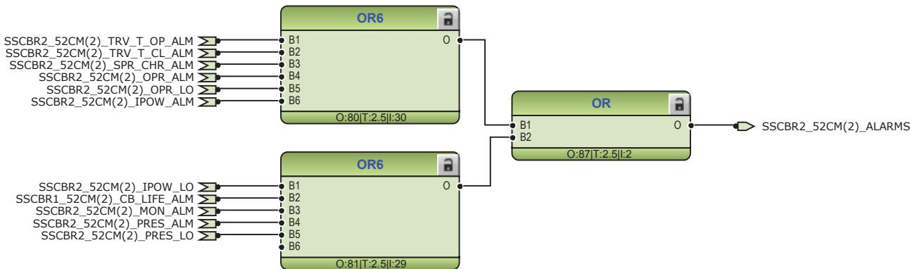
**Figure 30:** Logic for circuit breaker 2 monitoring alarm
