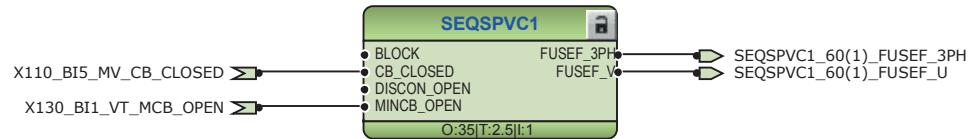
*Figure 79: High-voltage fuse failure supervision function*
