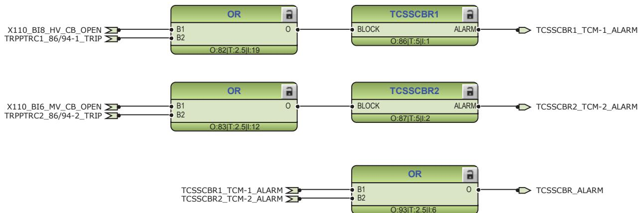
*Figure 84:* Trip circuit supervision function
