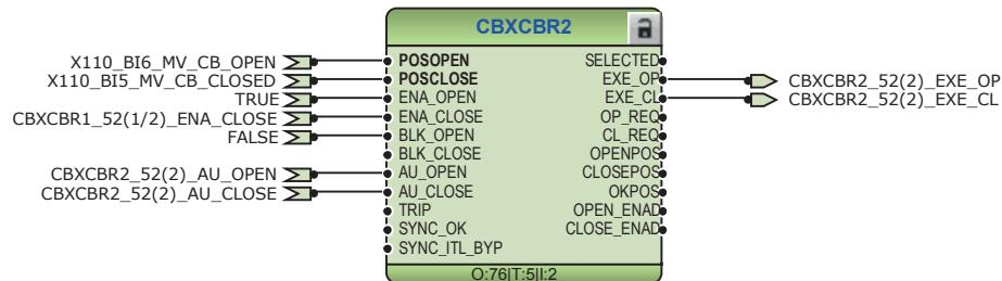
Figure 87: Circuit breaker 2 control logic
