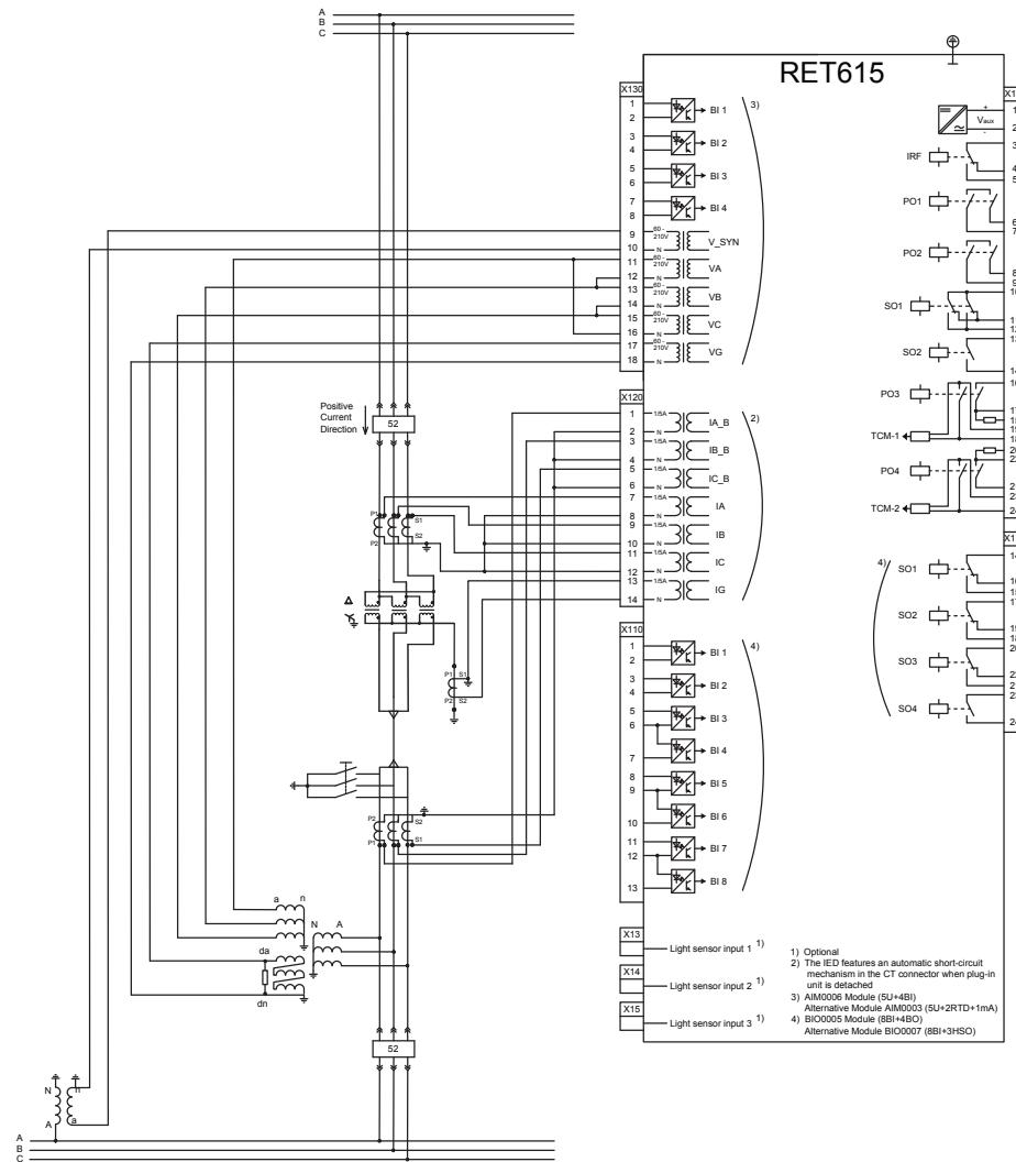
Figure 10: Connection diagram for the F configuration
