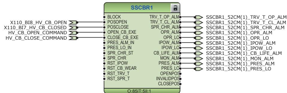
*Figure 80: Circuit-breaker 1 condition monitoring function*
