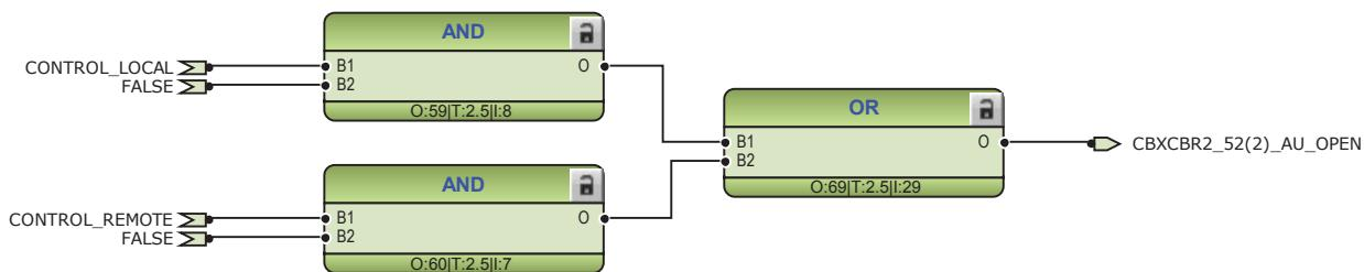
Figure 96: External opening command for circuit breaker 2
