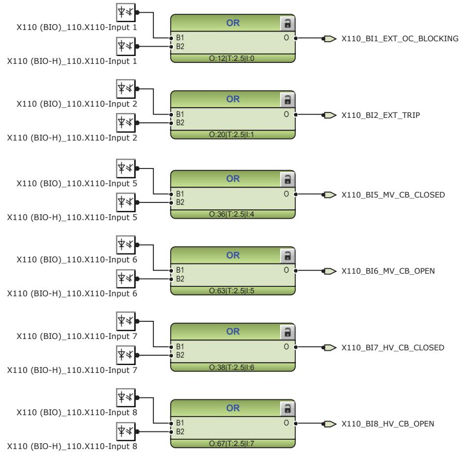
Figure 51: Default binary inputs - X110
