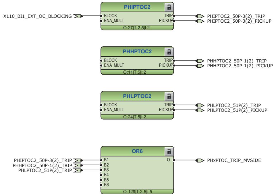
*Figure 65: Medium-voltage side overcurrent protection function*
