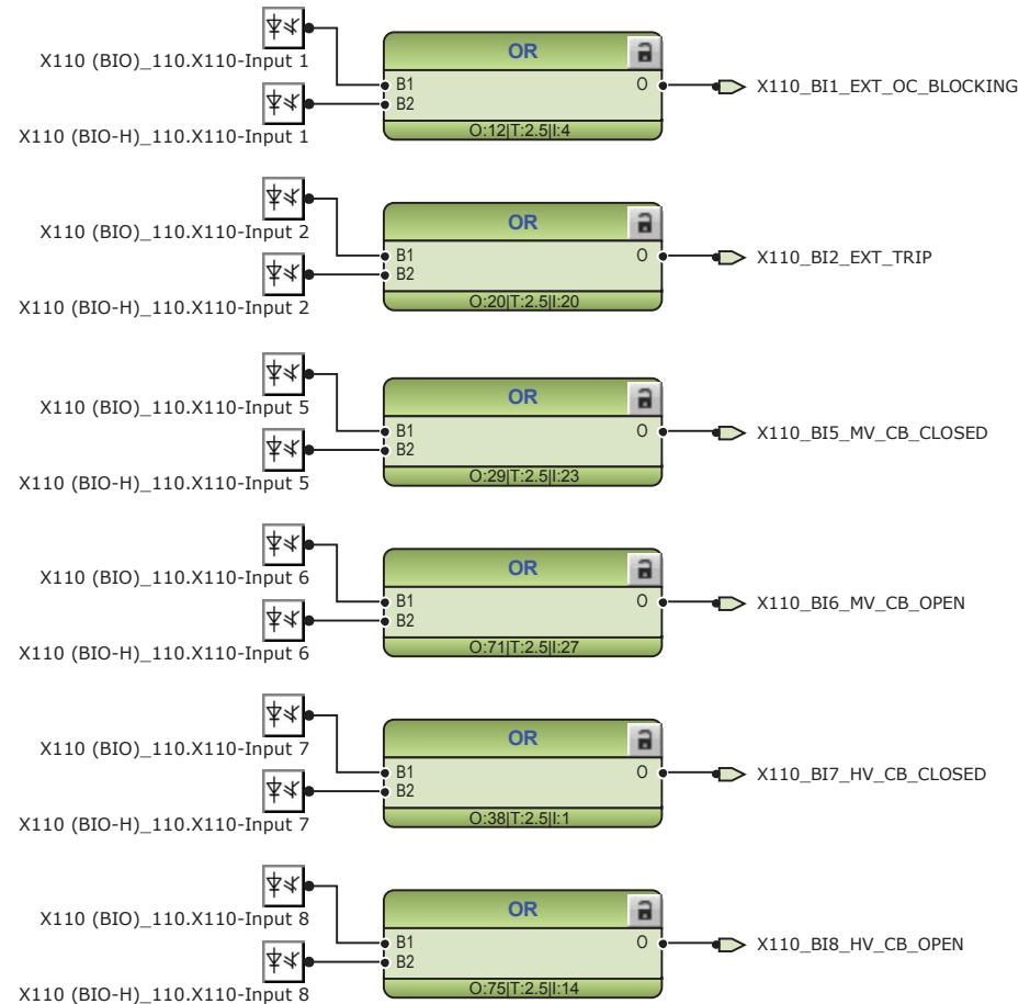
Figure 108: Default binary inputs - X110
