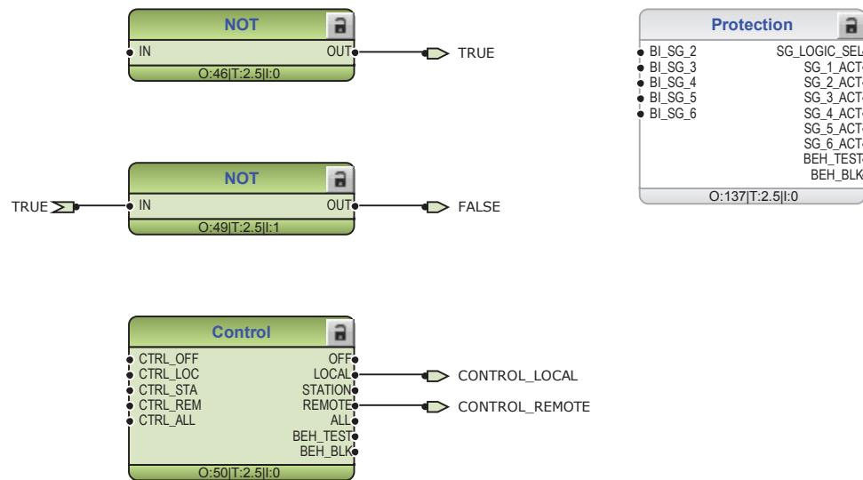
Figure 57: Functions for general logic states TRUE and FALSE, protection setting group selection and local and remote control
