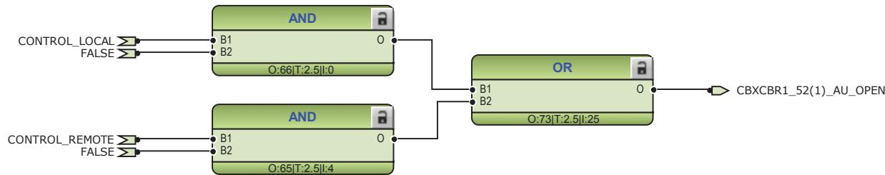
Figure 95: External opening command for circuit breaker 1
