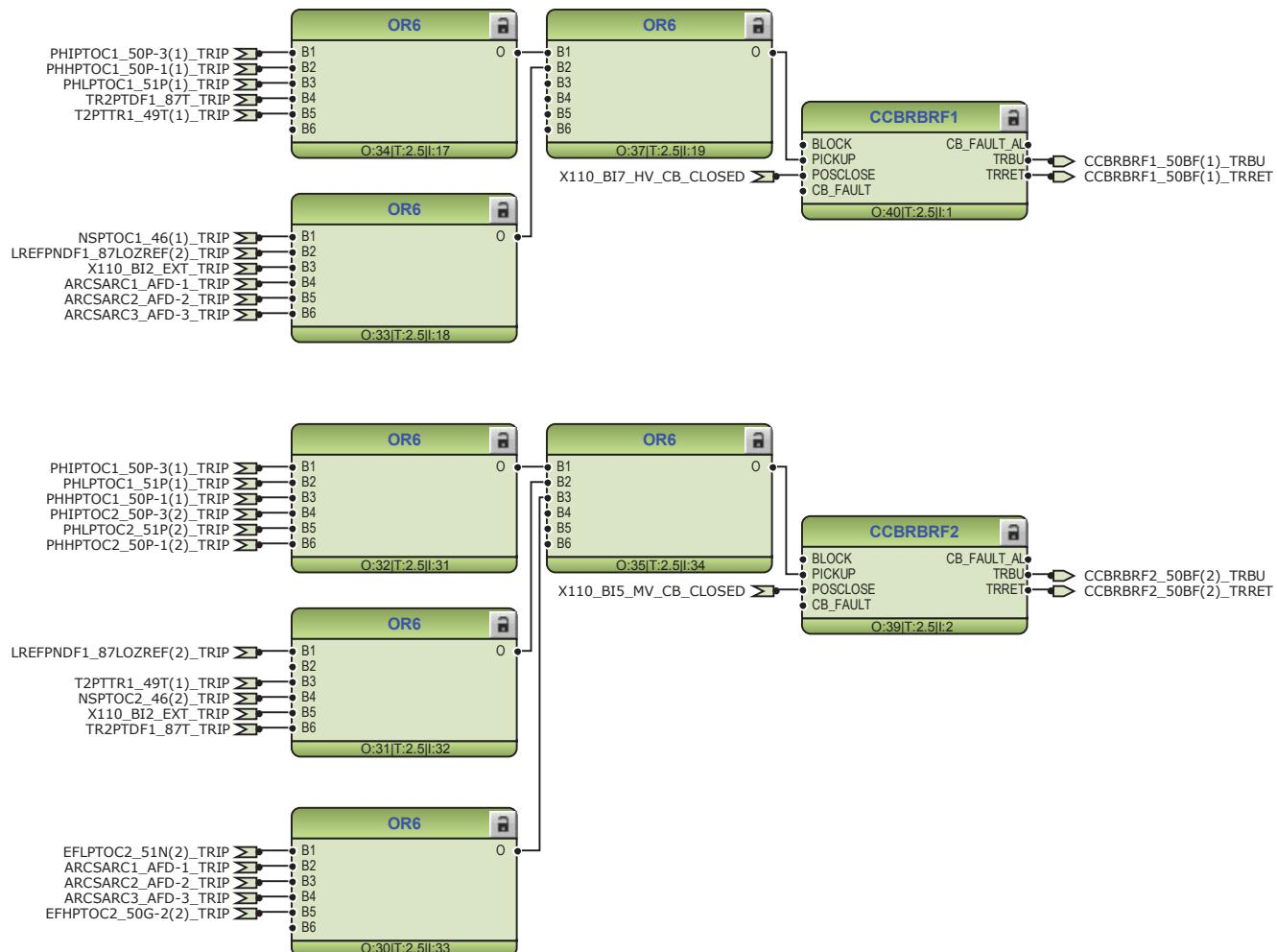
Figure 20: Circuit breaker failure protection function
