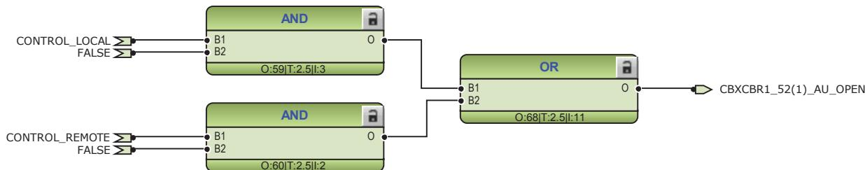
*Figure 41: External opening command for circuit breaker 1*
