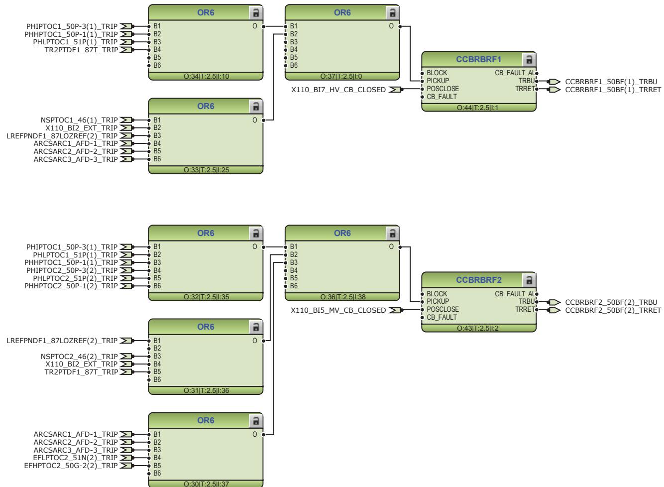
Figure 70: Circuit breaker failure protection function
