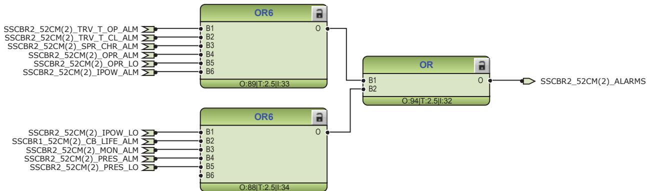
Figure 83: Logic for circuit 2 breaker monitoring alarm
