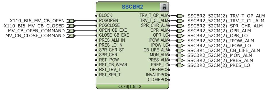
Figure 28: Circuit-breaker 2 condition monitoring function
