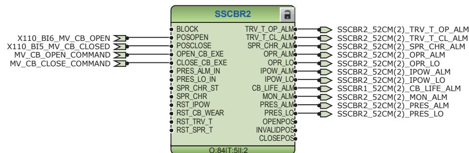
*Figure 81: Circuit-breaker 2 condition monitoring function*
