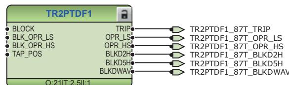
Figure 63: Transformer differential protection function
