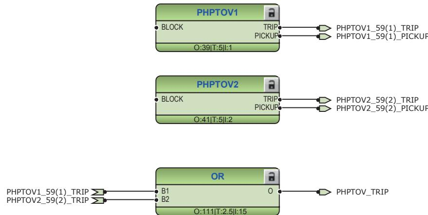
Figure 71: High-voltage side phase overvoltage protection function
