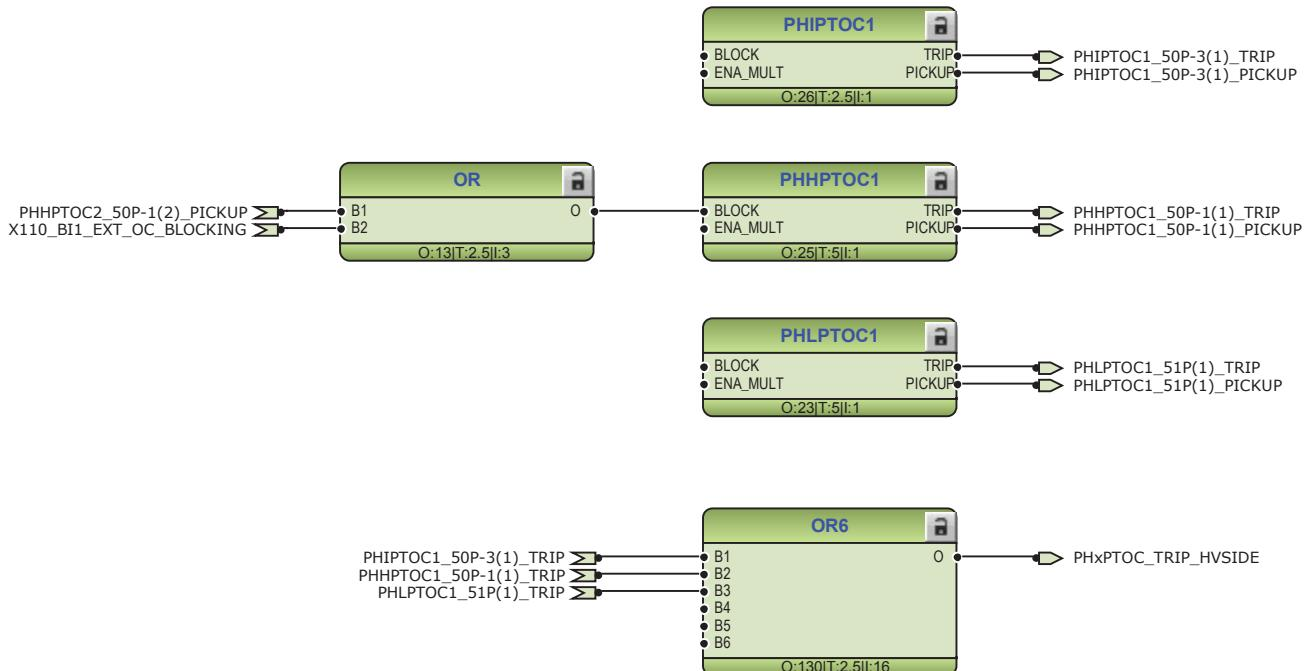
*Figure 64: High-voltage side overcurrent protection function*
