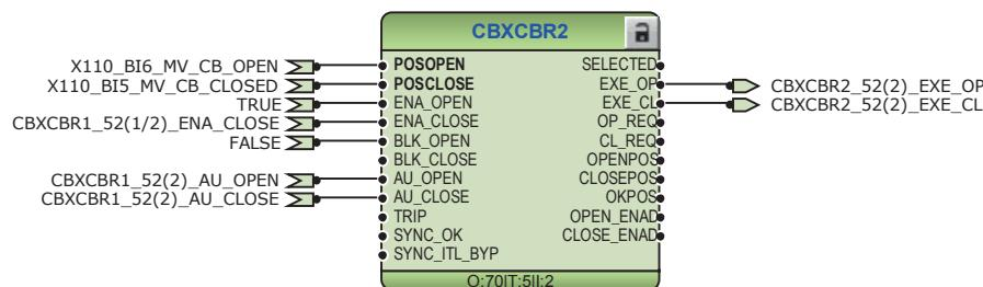
*Figure 33:* Circuit breaker 2 control logic
