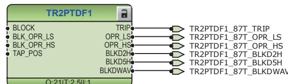
*Figure 12: Transformer differential protection function*
