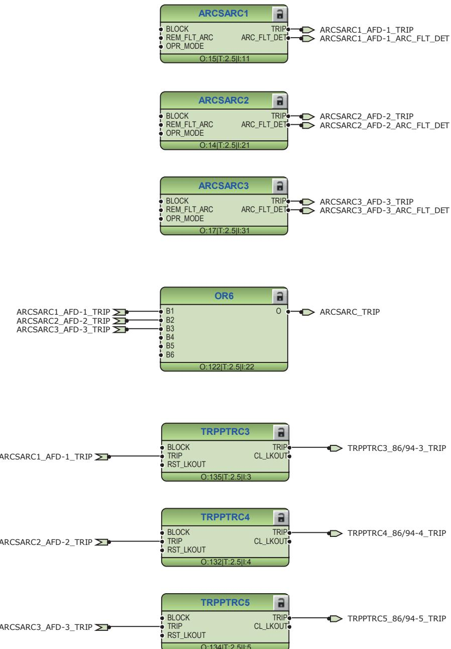
Figure 21: Arc protection with dedicated high-speed output
