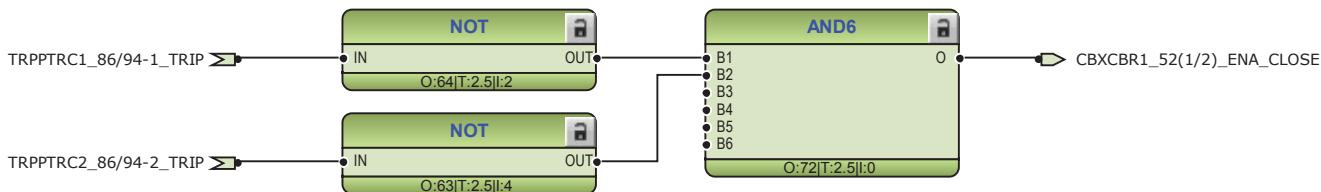
*Figure 92: Circuit breaker close enable logic*
