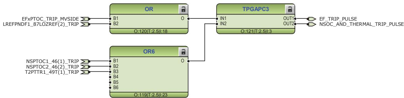
*Figure 59: Timer logic for ground-fault and negative sequence with thermal overload protection trip alarm*
