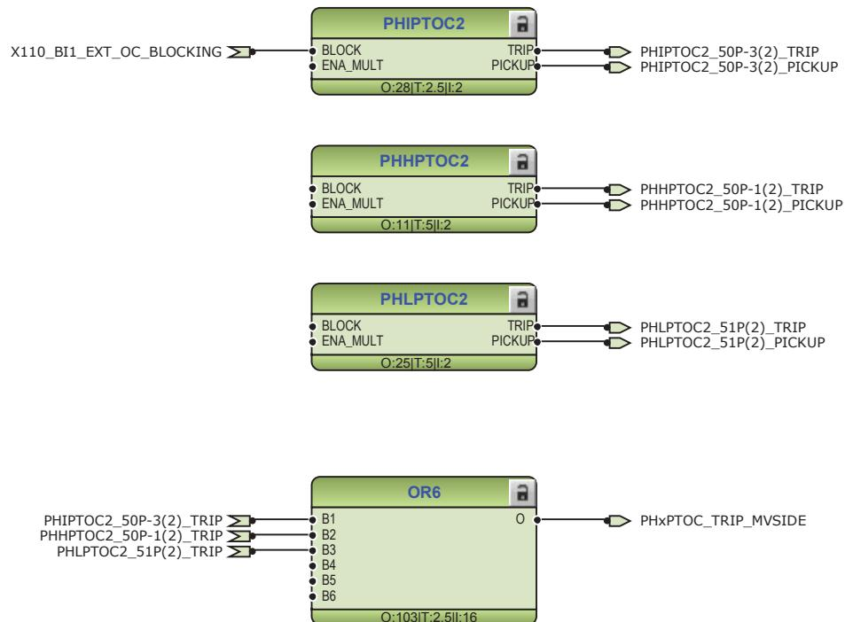
Figure 14: Medium-voltage side overcurrent protection function
