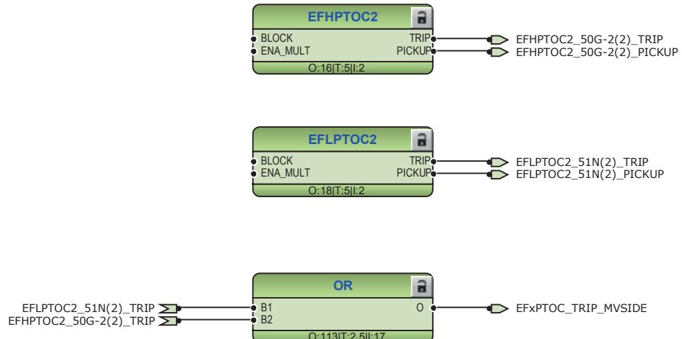
*Figure 66: Medium-voltage side ground-fault protection function*
