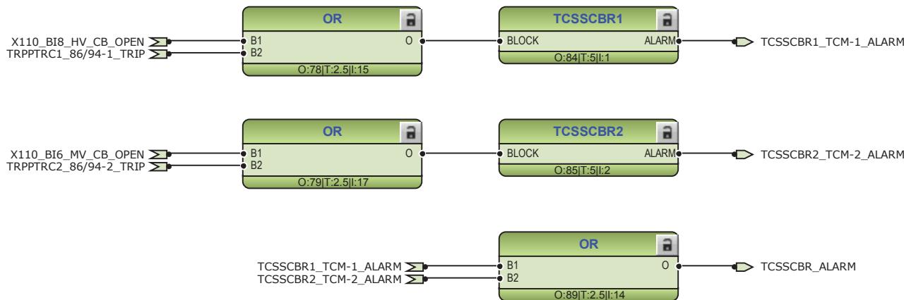
Figure 31: Trip circuit supervision function
