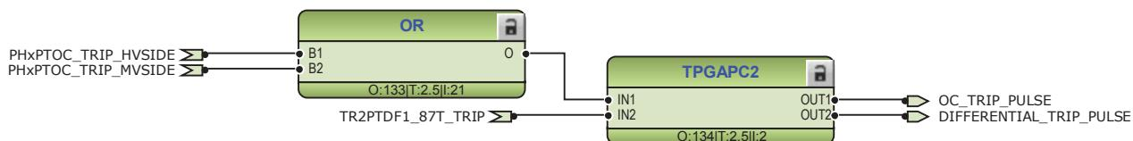
Figure 115: Timer logic for overcurrent and differential trip pulse
