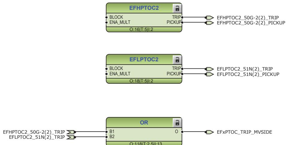
Figure 15: Medium-voltage side ground-fault protection function
