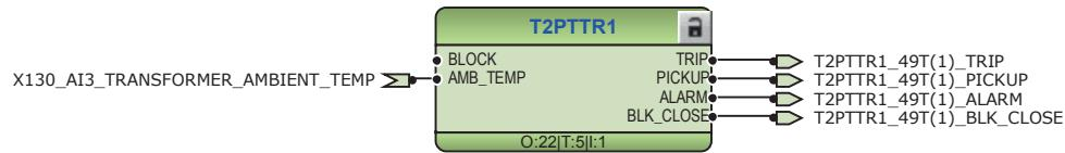
*Figure 19: Thermal overload protection function*
