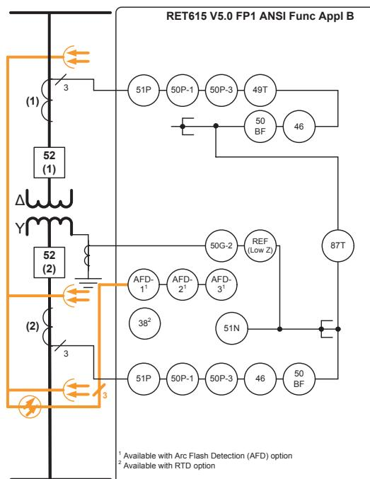
Figure 11: Functionality overview for standard configuration B
