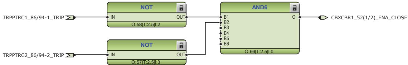
*Figure 38: Circuit breaker close enable logic*
