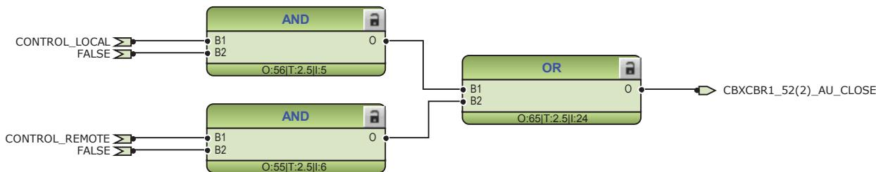
*Figure 40: External closing command for circuit breaker 2*
