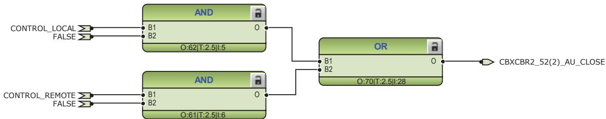
Figure 94: External closing command for circuit breaker 2
