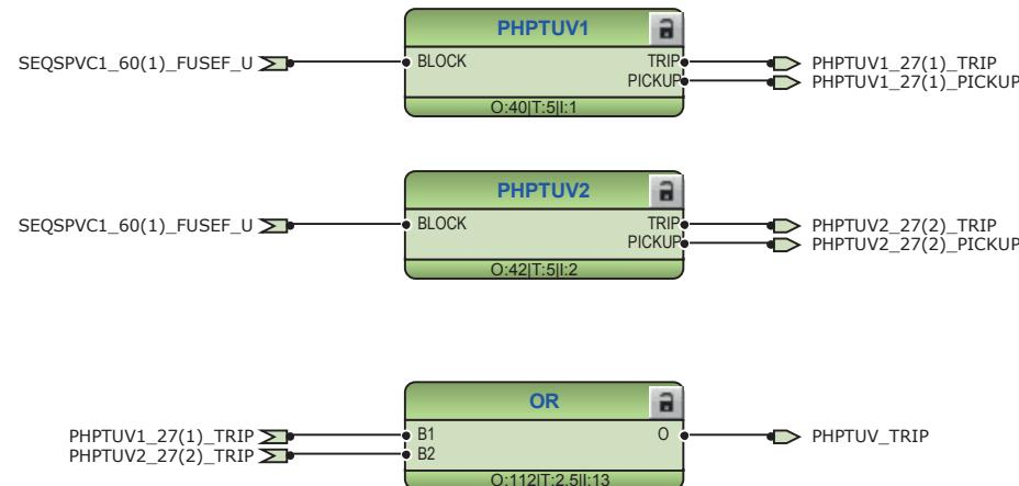
Figure 72: High-voltage side phase undervoltage protection function
