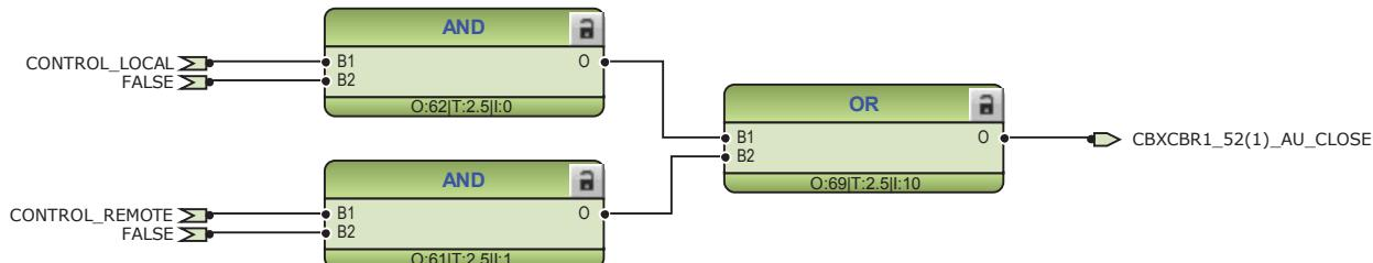
*Figure 39: External closing command for circuit breaker 1*
