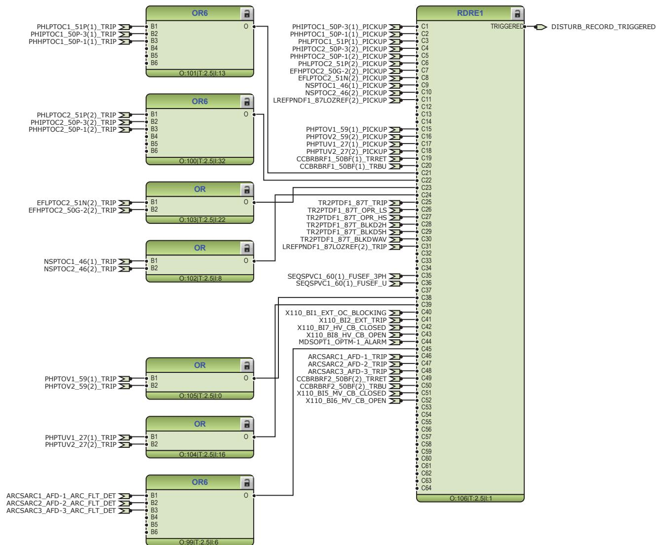
Figure 78: Disturbance recorder
