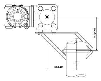
• 621ES transmitter with welded flanges on bracket for wall mounting (by four M8 screws)
