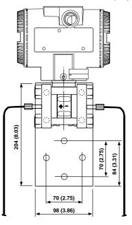
624ES transmitter on bracket for 60 mm (2in) pipe mounting (barrel housing)
