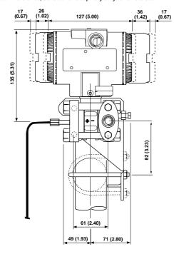
NOTE : For 621ES side with 1/2"-14 NPT threaded process flange connection, gasket groove and gaskets are in accordance with DIN 19213; removing adapter the flange provides a direct 1/4"-18 NPT thread. Bolting threads for fixing adapter or other devices (i.e. manifold etc.) on process flange is 7/16"-20 UNF.
