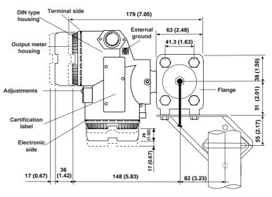
• 621ES transmitter with welded flanges on bracket for vertical or horizontal 60 mm (2in) pipe mounting
