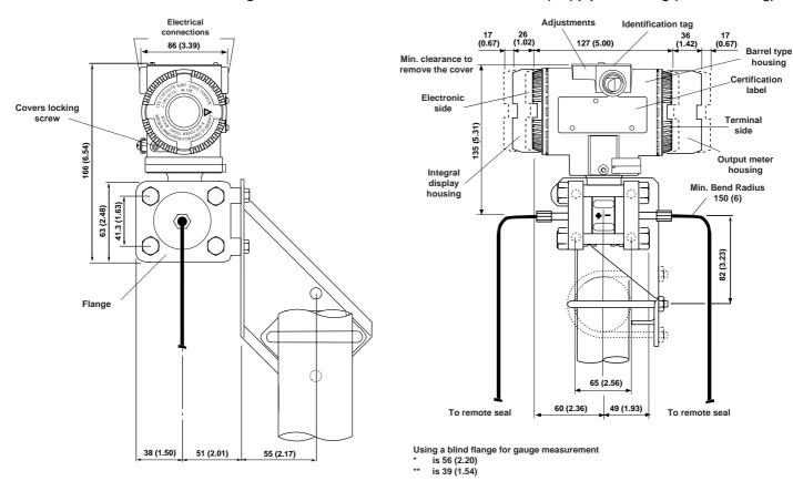
Dimensions of positive and negative side can be inverted according to high and low pressure side code selections. Selecting one side with blind flange (for gauge) or vacuum reference, consider one capillary only to remote seal
