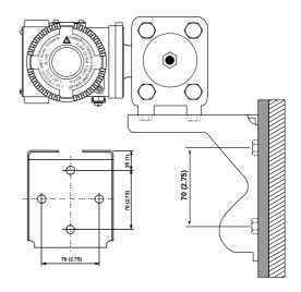
• 621ES transmitter with welded flanges on flat type (for box) bracket for vertical or horizontal 60 mm (2in) pipe mounting
