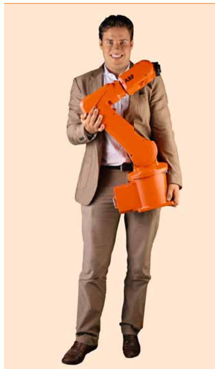
2 The IRB 120 weighs in at 25 kg
