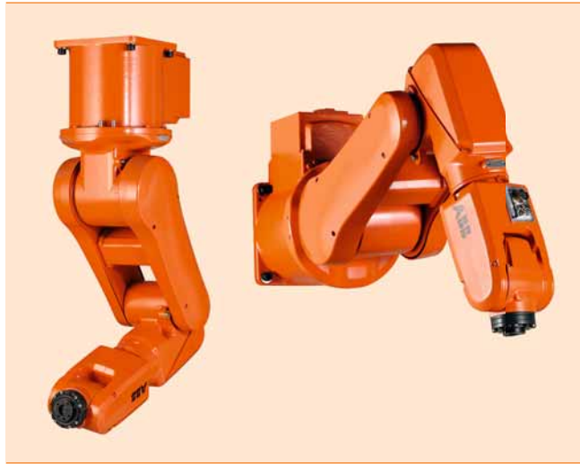
1 The IRB 120 can be mounted in a wide range of positions. Here, it is mounted from the ceiling (left) and a wall (right).
